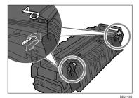
Holding the fusing unit by the handles, carefully push the fusing unit into the printer completely.
