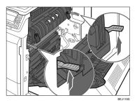
2. Holding the fusing unit by the handles, slowly pull out the fusing unit until it stops.
