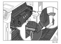
**4.** Holding the fusing unit firmly by the handles, pull out the fusing unit completely.
