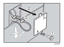
Fasten the band as shown until it clicks to secure the cable.
