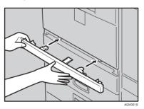
Pull the second paper tray (Tray 2) until it stops. After that, lift it slightly, and then pull it out.
