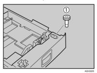
E Lock the Paper Bank and the printer with the screw.
