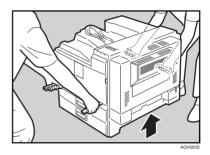
Push the grips into the printer. Take out the cover inside Tray 2 and attach it between the paper tray and the front cover.
