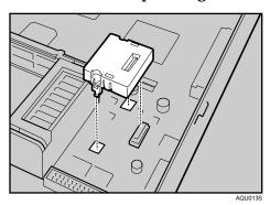
Make sure that User Account Enhance Unit is firmly connected to the controller board.
