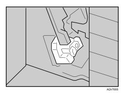
The cartridge compartment is located at the bottom of the finisher.
