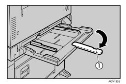
2 Slide the paper guides outwards, and then load paper until it stops with the print side down.
