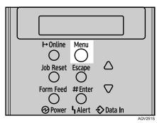
Select [Host Interface] using [▼] or [▲], and then press the [# Enter] key.
