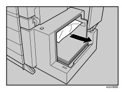
If you cannot remove the misfed paper in the previous step, close the top cover of the Large Capacity Tray RT45 and pull the lever (1) to extend the connecting unit (2).
