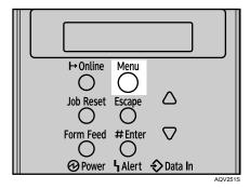
**2** Select [Paper Input] using [▼] or [▲], and then press the [# Enter] key.
