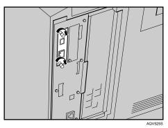
Check the Gigabit ethernet board is connected firmly to the controller board.
