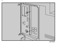
**5** Hold the part (1) of the controller board, and then slide it out completely.
