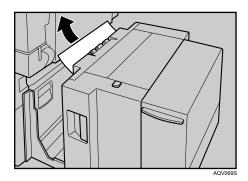
**5** Slide the Large Capacity Tray RT45 forward to connect it to the printer.
