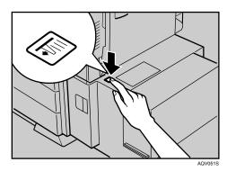
2 When the button stops blinking and is lit, open the top cover.
