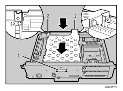
Fasten the screws clockwise as shown by using the provided screwdriver, to secure the hard disk drive.
