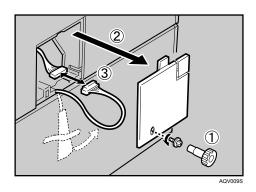
**P** Fasten the band as shown until it clicks to secure the cable.
