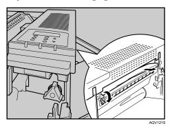
Turn the blue knob B counterclockwise (1), and then remove the misfed paper from inside the right cover (2).
