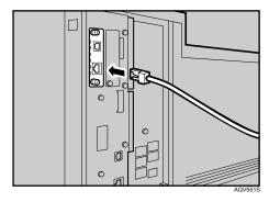
3 Connect the other end of the cable to the printer's network, such as a hub.
