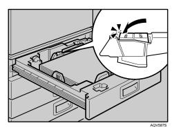
Adjust the paper size dial to match the size and feed direction of the paper in the paper tray.
