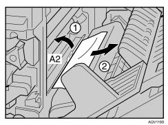
Open the Bypass Tray, and then remove the misfed paper.
