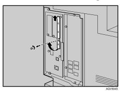
**1** Carefully insert the VM card into the slot, until the card clicks into place.
