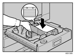
Confirm that the top of the stack is not higher than the limit mark inside the tray.
