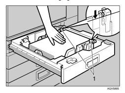
The rear guide is not necessary when  $11 \times 17$  inch paper is loaded in the tray. Put it in the holder in the tray.
