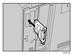
Confirm that the 1284 interface board is firmly connected to the controller board.
