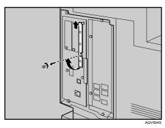
**4** Carefully insert the data storage card into the slot, until the card clicks into place.
