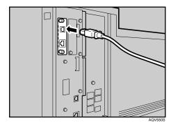
The printer's ethernet and USB ports are not available when the gigabit ethernet board is attached to the printer.
