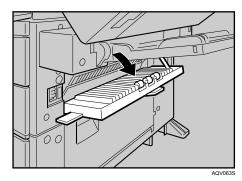
If your printer is equipped with the optional Large Capacity Tray RT45, the upper vertical paper feed cover is removed.
