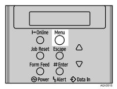
**2** Select [Maintenance] using [▼] or [▲], and then press the [# Enter] key.
