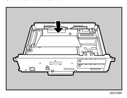
Connect the flat cable (1) and power cable (2) to the hard disk drive.
