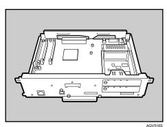
Remove the default or optional SDRAM module before installing the hard disk drive. Press down the levers on both sides (1) to remove the SDRAM module (2).
