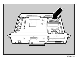
**8** Align the notch of User Account Enhance Unit, and then insert it into the controller board, pressing it down until it clicks into place.
