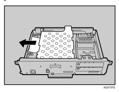
Be sure to check whether the hard disk drive is completely secured before removing the sheet.
