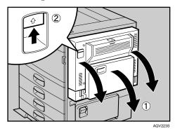
**3** Open the right cover by pushing the catch upwards.
