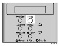
**2** Select [Host Interface] using [▼] or [▲], and then press the [# Enter] key.
