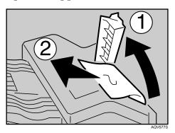
2 If you cannot remove misfed paper, open the slide cover and remove the misfed paper.
