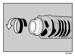
After removing the black cap from the bottle, toner can scatter easily. Do not shake or jar the bottle.
