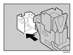
Align the arrows on the new refill and the cartridge, and then push in the refill until it clicks.
