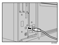
2 If the gigabit ethernet board is attached, connect the square-shaped connector of the USB2.0 cable to the USB port of the board.
