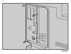
4 Hold the part (1) of the controller board, and then slide it out completely.
