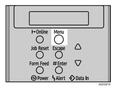
**2** Select [Paper Input] using [▼] or [▲], and then press the [# Enter] key.
