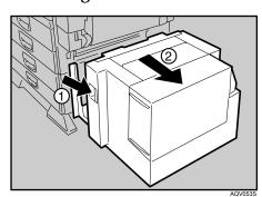
A Remove the misfed paper from the left side of the Large Capacity Tray RT45.
