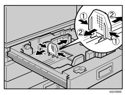
**E** Align all four sides of the paper stack and load it into the tray with the print side up.
