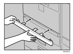
Pull the second paper tray (Tray 2) until it stops. After that, lift it slightly, and then pull it out.
