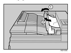
2 Open the Bypass Tray (1), and then open the Duplex Unit by pushing the catch upwards (2).
