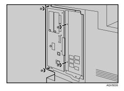
The printer may malfunction if the controller board is not properly installed.
