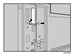
The removed cover is not used when installing the interface unit.
