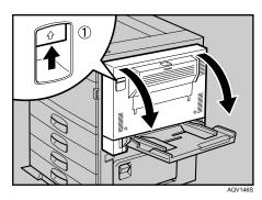
Open the cover Z to the left (1), and then remove the misfed paper (2).
