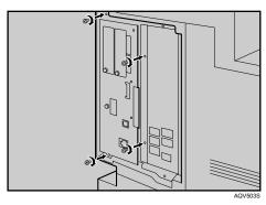
The printer may malfunction if the controller board is not properly installed.
