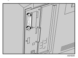
6 Attach the antenna to the card with the label facing down and the uneven side of the antenna facing up.
