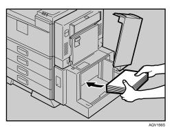
Confirm the top of the stack is not higher than the limit mark inside the tray.
