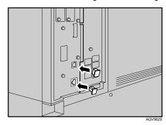
Remove the screw by turning it counterclockwise using the provided screwdriver, and then remove the cover of the Gigabit ethernet board slot.
