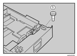
A Remove the screws as shown by turning them counterclockwise using the provided screwdriver.
