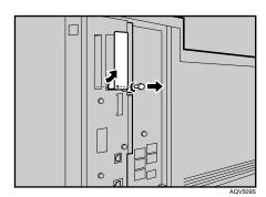
The removed cover is not used when installing the 1284 interface board.
