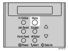
**2** Select [Maintenance] using [▼] or [▲], and then press the [# Enter] key.
