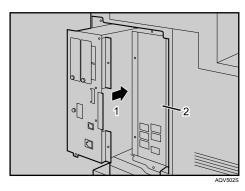
Push in the controller board firmly to align the rails in the printer's compartment.
