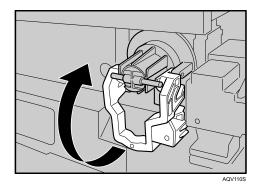
3 While pushing the lever to the right (1), hold the handle and gently slide the toner holder out (2).
