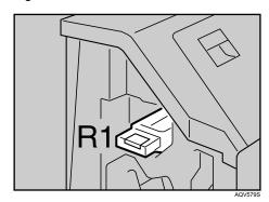
4 Hold up the lever R1, and remove the misfed paper.
