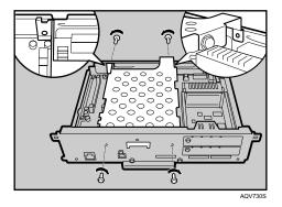
**P** Connect the power cable to the socket on the controller board.
