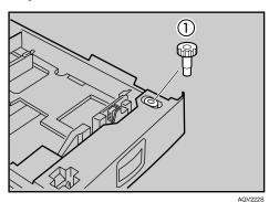
**1** Lock the Paper Bank and the printer with the screw.
