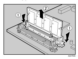
Be sure not to leave any SDRAM module in the slots. Doing so may damage SDRAM modules when installing the hard disk drive.
