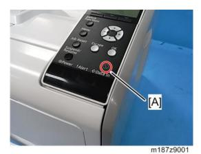
The ECO Night Sensor [A] (ambient light sensor) enables the printer to automatically turn off and on the main power when changes in the ambient light level are detected.
