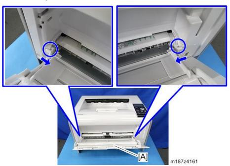
3. Release the hinges at both ends of by-pass tray [A] to detach it.
