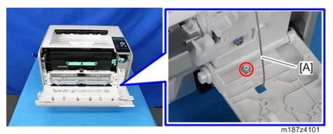
5. Release the hinges at both ends, and detach the front cover [A].
