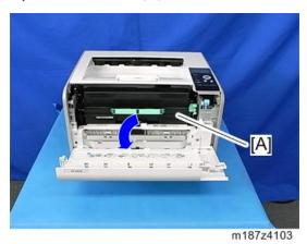
2. Two screws securing the front side of the left cover [A] (\$\mathbb{O}^{\mathbb{O}} \times 2)\$
