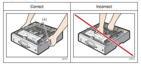
Be sure to lift the optional tray by holding the handles indicated by [A]. The tray may be damaged if you hold any parts other than the handles.
