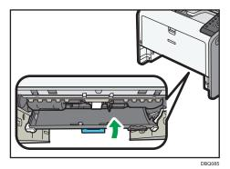
5. Lift the front side of the tray, and then slide it into the printer carefully until it stops.
