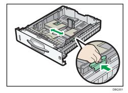
4. Squeeze the end guide and slide it inward to match the standard size.
