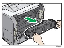
8. Hold the tab, and then remove the jammed paper.
