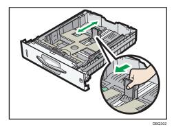
5. Slide the two levers at the bottom of the tray according to the thickness of the paper.
