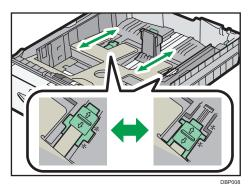
If the paper is heavier than  $130 \text{ g/m}^2$  (35 lb.), slide both levers into the rear (thick) position. If the paper is  $130 \text{ g/m}^2$  (35 lb.) or lighter, slide both levers into the forward (thin) position.
