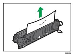
9. If the paper is not jammed in the fusing unit, remove the jammed paper from inside of the printer.
