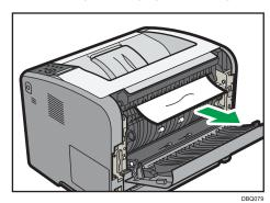
8. If you can see the jammed paper in the output tray, keep the rear cover opened and remove the paper.
