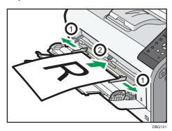
3. Adjust both sides of the paper guide to match the paper width.
