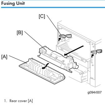
2. Fusing unit [B] (2 hooks [C])
