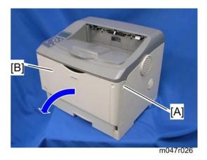
1. Press the button [A], and then open the front door [B].
