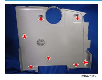
There are seven tabs on the right cover. Each arrow shows the direction of the tab.
