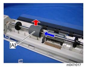
4. Slide the by-pass feed roller [A] to the left, and then remove it.
