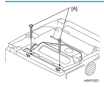
Use the scanner positioning pins (P/N: A0069104) to reinstall the unit. Set the positioning pins [A] as shown above. Then secure the laser unit.
