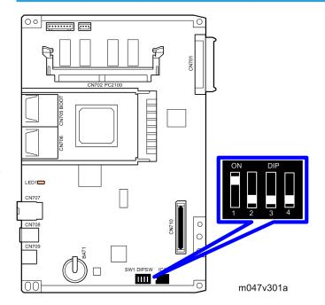
DIP Switch 1 (Bit 1) on the controller board is used for the error recovery after the firmware updating procedure failed.
