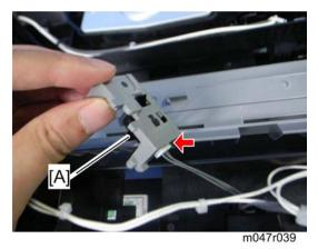
4. Fusing exit sensor [A] (hooks, 💷 x 1)
