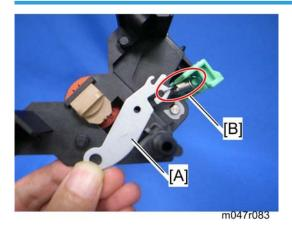
When attaching the pressure roller lever to the lower fusing unit assembly, attach the spring between the pressure roller lever and fusing unit first. If you try to attach the spring after attaching the pressure roller lever to the fusing unit, it is difficult to install the spring.
