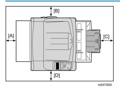
Place the machine near the power source, providing the clearance as shown below:
