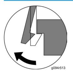
Many of the parts are held in place with plastic latches. The latches break easily, so release them carefully. To remove such parts, press the hook end of the latch away from the part to which it is latched.
