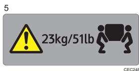
The printer weighs approximately 23kg (51 lb.). When moving the printer, use the inset grips on both sides, and lift slowly in pairs.
