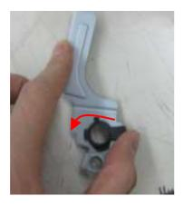
19. Remove the pressure roller bushing.
