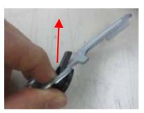
21. Rotate the new bushing to fix it in place.
