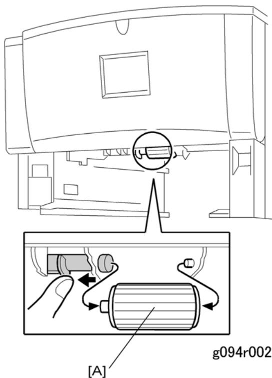
1. Pull out the paper tray before removing the paper feed roller.
