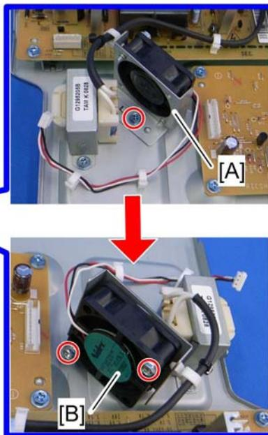
4. PSU fan with the bracket [A] (⚙️ x 1, 🛠️ x 2)
