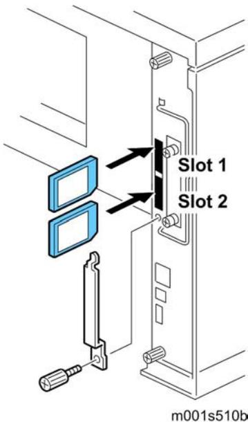
2. Remove the SD card slot cover.
