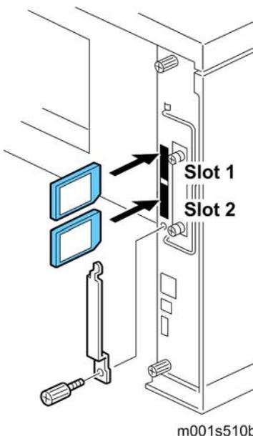
2. Remove the SD card slot cover.
