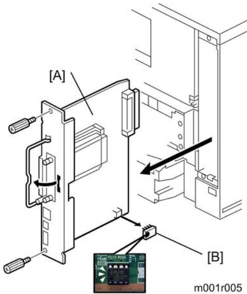
1. Printer controller board [A] (⚙️ x 2)
