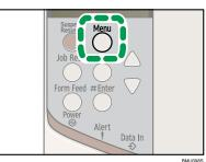
Press the [V] or [A] key to display [List/Test Print], and then press the [# Enter] key.
