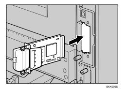
5. Fasten the wireless LAN interface unit to the controller board with the two screws.
