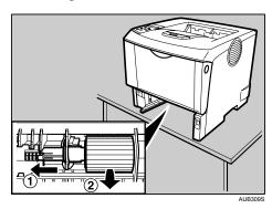
7. Wipe the rubber part of the roller with a soft damp cloth. Then, wipe it with a dry cloth to remove the water.
