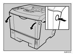
2. Lift the front side of the toner cartridge, and then pull it out of the printer.
