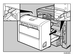
2. Lift the guide board inside the duplex unit, and remove the misfed paper.
