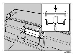
After pushing in the friction pad, press on it several times to check it is properly installed. If it jumps back into position due to the force of the spring, it is properly installed.
