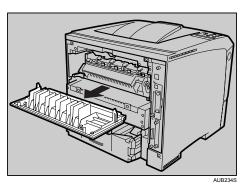
5. If the optional duplex unit is attached, push down the lever on the right side of the duplex unit (1), and then pull it out until it stops (2).
