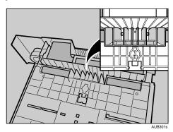
The friction pad may fall off when the catches are released. Place your hand over the friction pad while releasing the catches.
