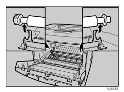
6. Insert the new transfer roller on the socket with the gear of the roller positioned to the left.
