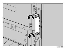
The removed cover is not used when installing the wireless LAN interface unit. Keep it for possible future use.
