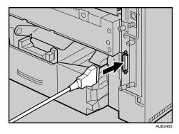
3. Securely attach the other end of the parallel cable to your computer's parallel port. Secure the cable.
