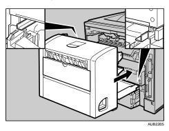
15. Securely push the duplex unit into the printer.
