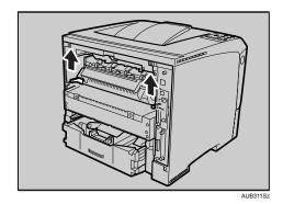
6. Pull the fusing unit out.
