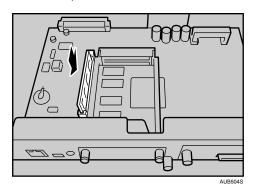
6. Replacing the default SDRAM module, press down the levers on both sides (1) to remove the default module (2).
