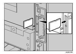
5. Reattach the cover over the optional card. Fasten the screw to secure the cover.
