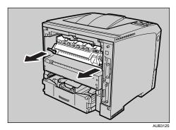
7. Pull out the pins on both sides of the new fusing unit.
