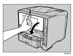
2. If the optional duplex unit is attached, push down the lever on the right side of the duplex unit (1), and then pull it out until it stops (2).
