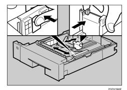
4. Push the bottom plate down until it locks into place.
