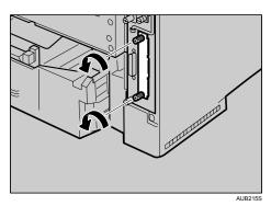
The removed screws and cover are not used when installing the hard disk drive.
