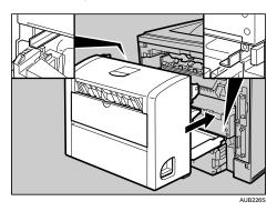
7. Securely push the duplex unit into the printer.
