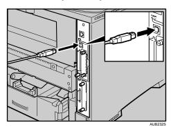
2. If the Gigabit Ethernet board is attached, connect the square-shaped connector of the USB2.0 cable to the USB port of the board.
