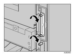
Check the wireless LAN interface unit is connected firmly to be controller board.
