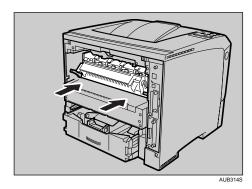
9. Push the lock levers of the fusing unit down until they click.
