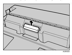
6. Insert the new friction pad in the paper tray.
