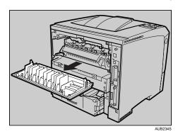
3. If the optional duplex unit is attached, push down the lever on the right side of the duplex unit (1), and then pull it out until it stops (2).
