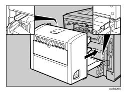
8. Push the duplex unit securely into the printer.
