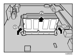
7. Align the notch of the SDRAM module to the slot, and then push it down until it clicks.
