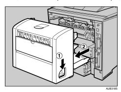
6. Push the under board levers (1) and then pull the duplex unit out of the printer (2).
