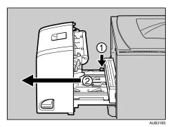
5. Lift the lock levers of the fusing unit as shown in the illustration.
