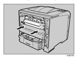
11. Push the lock levers of the fusing unit down until they click.
