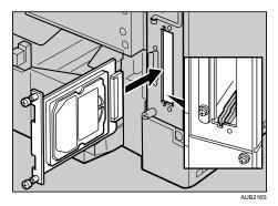
5. Fasten the two screws to fix the hard disk drive.
