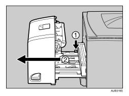
7. Lift the lock levers of the fusing unit as shown in the illustration.
