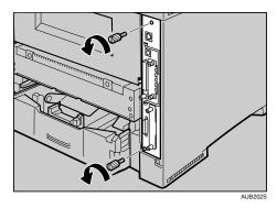
The removed screws are required in fastening the controller board.
