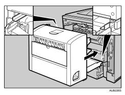
11. Securely push the duplex unit into the printer.
