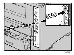
3. Connect the other end of the cable to the network, such as a hub.
