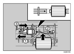
Confirm the green lock lever secures the roller correctly by checking that sure the new roller rotates smoothly.
