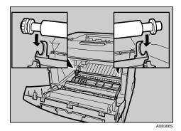
7. Push down the lock levers on both ends of the printer as shown in the illustration, until they click into place.
