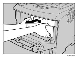
4. Wipe around the metallic Registration roller by turning with a soft damp cloth.
