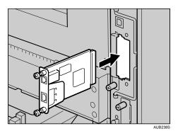
6. Fasten the Gigabit Ethernet board to the controller board with two screws.
