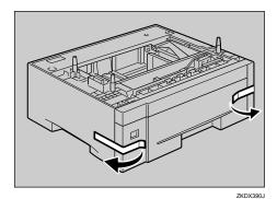
4. Align the holes over the pins, and then lower the printer gently onto the paper feed unit.
