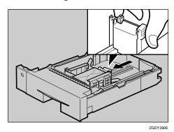
8. Lift the front of the tray, and then slide it carefully into the printer until it stops.
