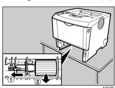
7. While sliding the green lock lever to the left  $(\mathbb{Q})$ , set the new roller  $(\mathbb{Q})$ . Then, return the green lock lever to its original position  $(\mathbb{Q})$ .
