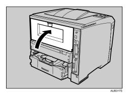
12. When the optional duplex unit was removed, push in the duplex unit along the rails in the back of the printer.
