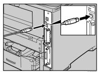
Connect the opposite end's flat connector to devices such as your computer's USB interface, or a USB hub.
