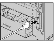
Securely attach the other end of the parallel cable to your computer's parallel port. Secure the cable.
