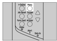
Press the [V] or [A] key to display [Host Interface], and then press the [# Enter] key.
