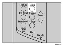
Press the [V] or [A] key to display [List/Test Print], and then press the [# Enter] key.
