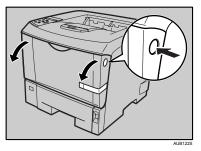
Remove the fixing material inserted between toner cartridge and the printer.
