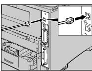
Connect the other end of the cable to the printer's network, such as a hub.
