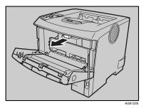
Lift the front side of the toner cartridge, and then pull it out of the printer.
