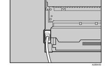
Insert the plug of the power cord securely into the wall outlet.
