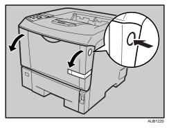
2 Remove the fixing material inserted between toner cartridge and the printer.
