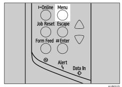
**3** Press the **(▼)** or **(△)** key to display [List/Test Print], and then press the [ # Enter] kev.
