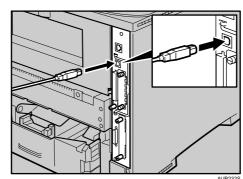
**2** Connect the opposite end's flat connector to devices such as your computer's USB interface, or a USB hub.
