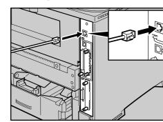
**2** Connect the other end of the cable to the printer's network, such as a hub.
