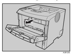
Lift the front side of the toner cartridge, and then pull it out of the printer.
