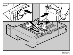
4. Push the bottom plate down until it locks into place.
