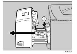
4. Push the under board levers (0), and then pull the duplex unit out of the printer (2).
