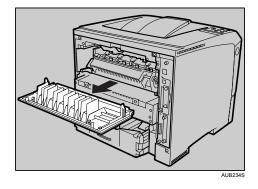
5. If the optional duplex unit is attached, push down the lever on the right side of the duplex unit (①), and then pull it out until it stops (②).
