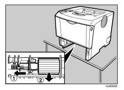
7. While sliding the green lock lever to the left (1), set the new roller (2). Then, return the green lock lever to its original position (3).
