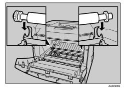
6. Insert the new transfer roller on the socket with the gear of the roller positioned to the left.
