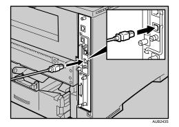
The printer's Ethernet and USB ports are not available when the Gigabit Ethernet board is attached to the printer.
