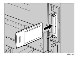
8. Attach the antenna cap to the card with the side that has both corners of the antenna cap cut out facing the screws.
