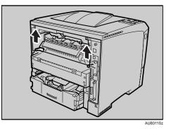
6. Pull the fusing unit out.
