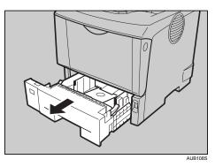
2. Lift the front side of the tray, and then pull it out of the printer.
