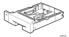
2. Pull out the optional paper tray (Tray 2) of the optional paper feed unit until it stops. After that, lift it slightly, and then pull it out.
