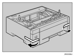
**4.** Align the holes over the pins, and then lower the printer gently onto the paper feed unit. There are three pins on the top of the paper feed unit that point straight up. On the bottom of the printer, there are three holes.
