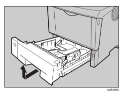
3. If the optional duplex unit is attached, push down the lever on the right side of the duplex unit (①), and then pull it out until it stops (②).
