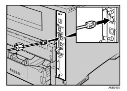
3. Connect the other end of the cable to the network, such as a hub.
