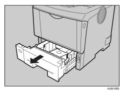
4. Lift the front side of the tray, and then pull it out of the printer.
