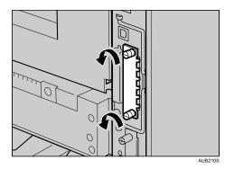
The removed cover is not used when installing the Gigabit Ethernet board. Keep it for possible future use.
