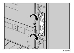
6. Fasten the Gigabit Ethernet board to the controller board with two screws.
