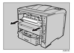
7. Pull out the pins on both sides of the new fusing unit.
