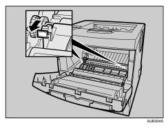
5. Hold the green parts of the roller on both sides, and remove the roller from the printer, as shown in the illustration.
