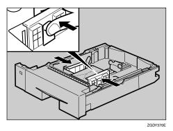
7. Pinch the rear guide, and then slide it along the edge of the envelope stack.
