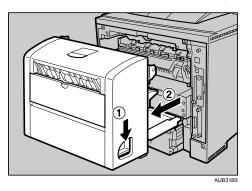
6. Push the under board levers (heta) and then pull the duplex unit out of the printer (heta).
