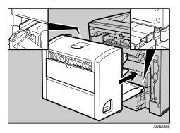
15. Securely push the duplex unit into the printer.
