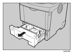
2. Lift the front side of the tray, and then pull it out of the printer.
