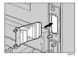
5. Fasten the IEEE 802.11b interface unit to the controller board with the two screws.
