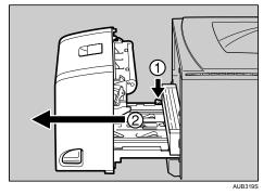
4. Push the under board levers (①), and then pull the duplex unit out of the printer (②).
