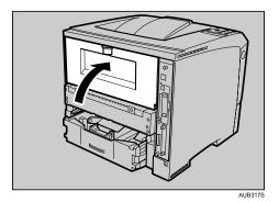
6. When the optional duplex unit was removed, push in the duplex unit along the rail in the back of the printer.
