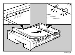
5. Lift the front of the tray, and then slide it carefully into the printer until it stops.
