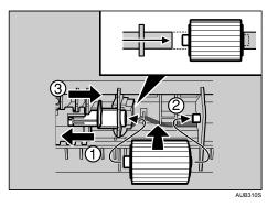
Check the green lock lever secures the roller correctly by making sure the new roller rotates smoothly.
