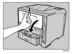
2. If the optional duplex unit is attached, push down the lever on the right side of the duplex unit (①), and then pull it out until it stops (②).
