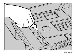
5. Load paper into the paper tray with the print side up. Carefully slide the paper tray into the printer until it stops.
