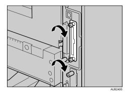
Check the IEEE 802.11b interface unit is connected firmly to be controller board.
