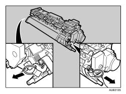
8. Push the new fusing unit into the printer.
