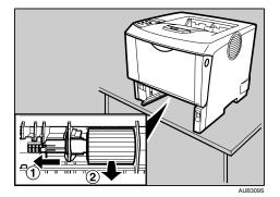
7. Wipe the rubber part of the roller with a soft damp cloth. Then, wipe it with a dry cloth to remove the water.
