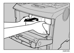
2. Lift the front side of the toner cartridge, and then pull it out of the printer.
