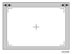
In this setting, adjust the margins of the test sheet so that they are equal in size.
