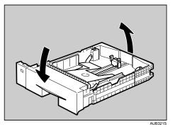
4. Use a sharp-pointed item like a ball-point pen, to release the two catches that lock the friction pad.
