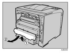
7. Push in the duplex unit along the rails at the back of the printer.
