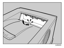
4. Open the front cover by pushing the front cover release button.
