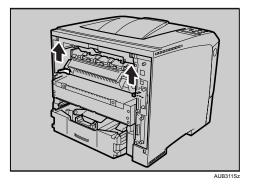
8. Pull the fusing unit out.
