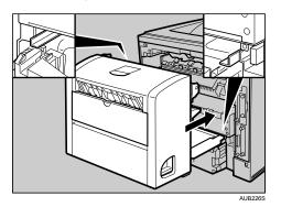
7. Securely push the duplex unit into the printer.
