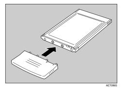
7. Insert the card slowly into the interface unit with the label facing down and the uneven black antenna surface facing up until it stops.
