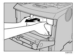
3. Pull the toner cartridge out of the printer by holding the grips of the cartridge.
