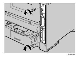
The removed screws are required in fastening the controller board.
