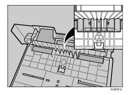
The friction pad may fall off when the catches are released. Place your hand over the friction pad while releasing the catches.
