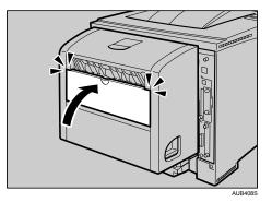
4. Lift the lever ( heta ), open the cover of the duplex unit ( heta ).
