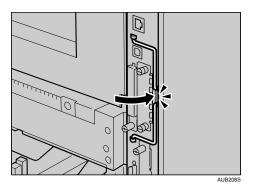
9. Fasten the controller board to the printer with the two screws.
