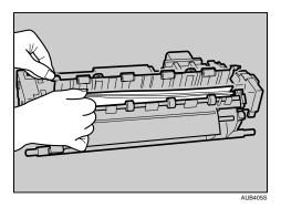
10. Push the fusing unit until it stops.
