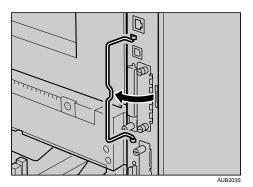
4. Pull the handle, and then slide the controller board out.
