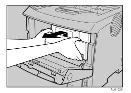
2. Pull the toner cartridge out of the printer, while raising the front side.
