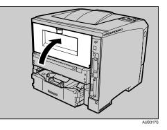
12. When the optional duplex unit was removed, push in the duplex unit along the rails in the back of the printer.
