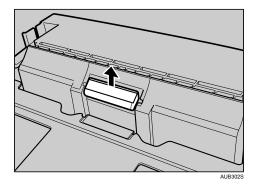
6. Insert the new friction pad in the paper tray.
