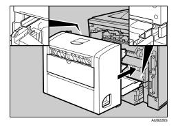
13. Securely push the duplex unit into the printer.
