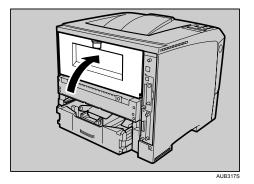
14. When the optional duplex unit was removed, push in the duplex unit along the rail in the back of the printer.
