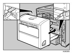
11. Securely push the duplex unit into the printer.
