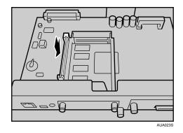
6. Align the notch of the SDRAM module to the slot, and then push it down until it clicks.
