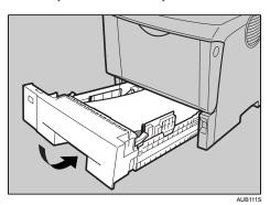
10. When the optional duplex unit was removed, push in the duplex unit along the rails in the back of the printer.
