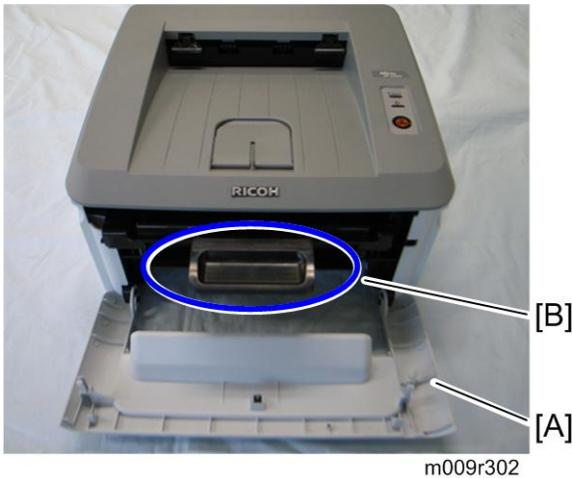
2. Remove carefully the front cover [A], using caution with the hooks.
