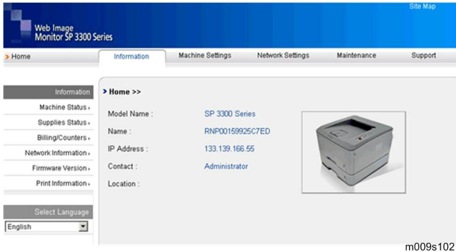
3. Access the "WIM" with the correct IP address.
