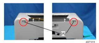
3. Press the tabs [A] on the top left and top right of the rear cover to detach the top of the rear cover.
