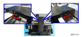
3. Push the carriage to the center, and then remove the top cover.
