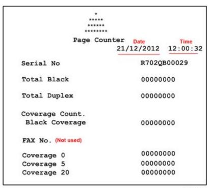
The counter lists the number of prints. The print totals do not include the number of test patterns that have been printed. The counter keeps totals for these items:
