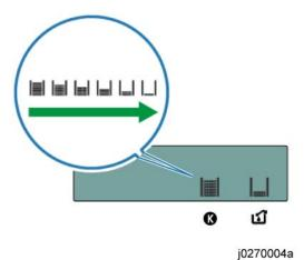
The printer shows a multi-level dynamic display that keeps the operator informed about the status of the ink levels in the tanks. The example below for Black (K) shows the progression in the display from full on the left to completely empty on the right.
