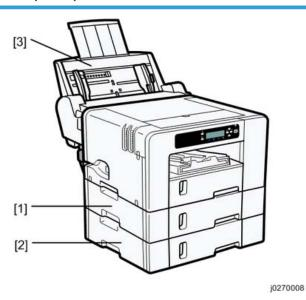
The Paper Feed Unit TK1160 (J312) is used with the J028/J029/J035. One [1] or two [2] paper feed units can be installed.
