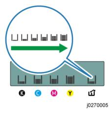
The amount of waste ink in the ink collector unit is indicated on a six-step scale, namely 0, 20, 40, 60, 80, and 100%. It is reset to 0% if a new ink collector unit is installed. If it reaches 100%, printing cannot be done. A message prompting the user to replace the unit appears on the panel display. A message prompting the user to replace the ink collector unit appears also if it is not mounted.
