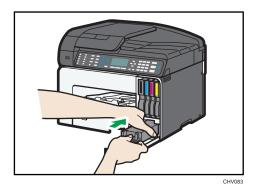
6. Slide the ink collector unit carefully into the machine until you hear it click.
