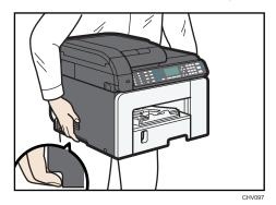
Grip the indented area at the base of the machine's sides, as shown. Lift and carry the machine slowly and carefully.
