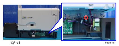
6. Remove the tension pulley unit. [A]
