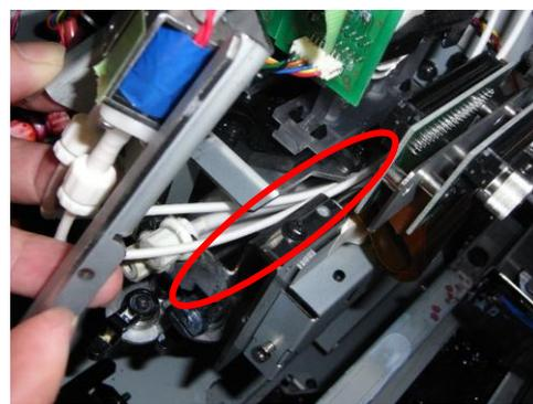
8. Put the circulation valve bracket back in place then fasten it down with screws. And set the connectors.
