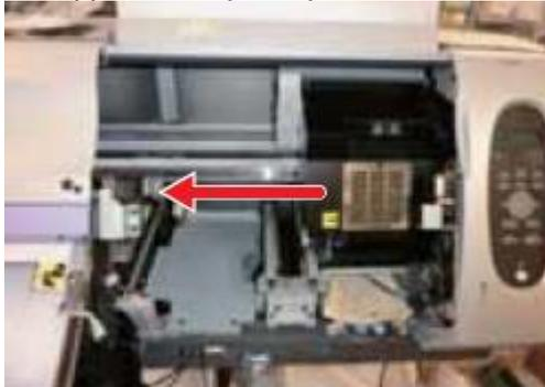
4. Remove the Cap ass'y. (Screw x4)
