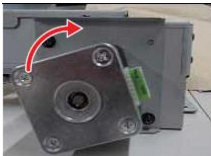
16. Press down as you attach the Wiper ass'y. (Screw x4)
