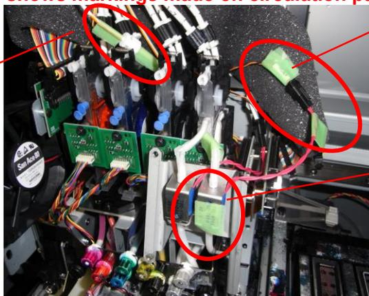
Mark both ends of the harness connector of the right solenoid with tape.
