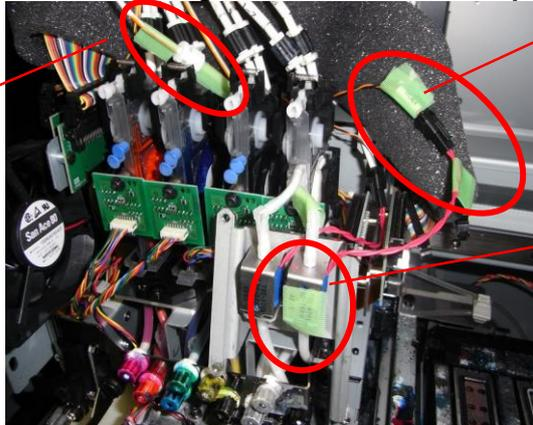
Mark both ends of the tube joint of the right solenoid with tape.
