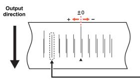
The dots at the fourth position counted from the zero position in the positive direction form a straight line. In this case, the dot position correction value is 4.0.
