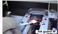
Space between the wiper slider and ink guard W
