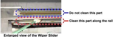
Enlarged view of the Wiper Slide and Ink Guard W
