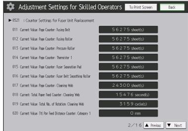
**52. Check the number appearing in [Current Value: Page Counter: Cleaning Web] and record it in the field next to "#0521 017" on the decal affixed on the fuser unit that was removed.**
