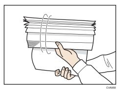
2. Holding its shorter ends, flex the stack back and forth to create space between the sheets. Repeat this several times.
