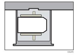
If you are printing onto side-opening envelopes, be sure to unfold their flaps and set them in the D orientation with print side face up. Flaps must be at the right side of the Wide LCT or multi bypass tray (Tray A).
