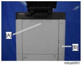
4. Tilt the operation panel [A] to a vertical position and remove the cover [B].
