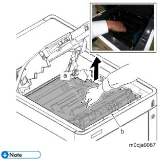
• Hold the handle (b) at the machine front side and lift up the ITB unit (a). Then, further lift it up
