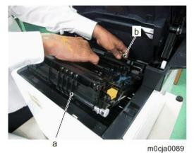
• Do not touch the release lever (b) after detaching the ITB unit (a).
