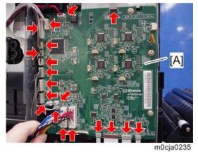
5. Release the wire from the hooks of the wire guide [A] and remove the wire guide [A] from the
