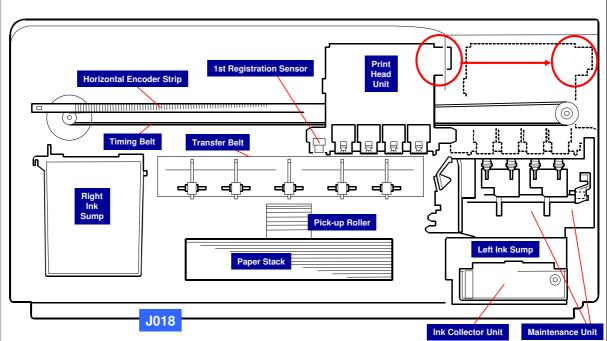
□ Note that Print Head Unit moves completely across picture above - from left to right and back, with resting place over Maintenance Unit, where the heads are capped to prevent them from drying out.
