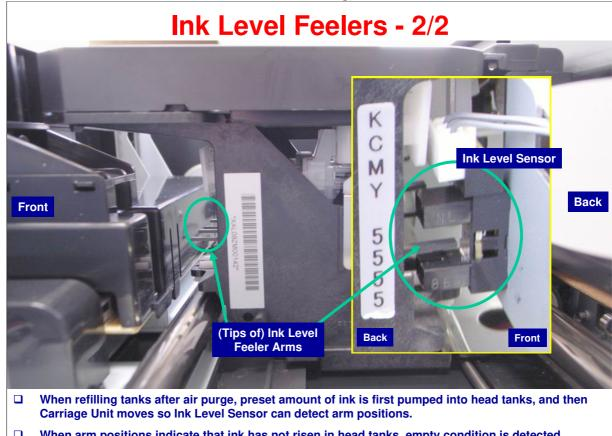
$f \square$  When arm positions indicate that ink has not risen in head tanks, empty condition is detected. Slide 60
