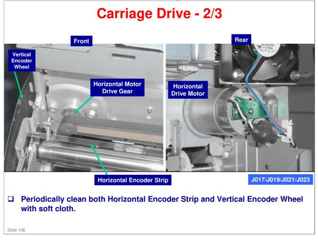
The Vertical Encoder Wheel is also known as the "Sub-scan Encoder Wheel".
