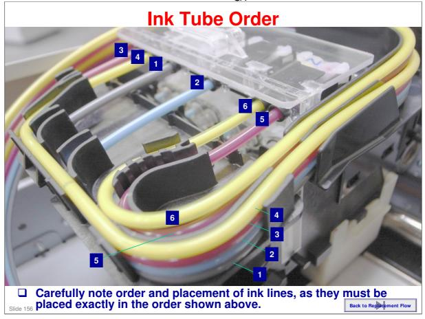
Note: Be certain that there is no pressure on the connections when installing a new lnk Carriage Unit – if there is, the ink lines could become detatched.
