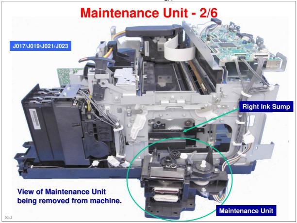
Maintenance unit above is from the  $J017/J019 \mod -$  the  $J018 \mod$  is slightly different.
