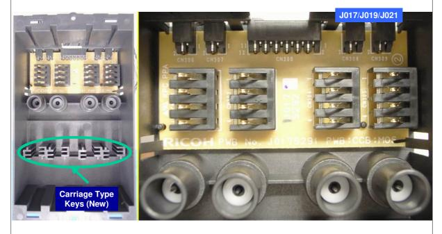
□ New shape Carriage-type Keys prevent older style cartridges from being used (and new type cartridges from being used in older machines).
