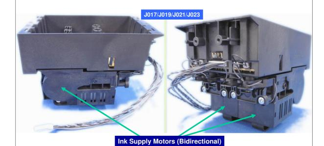
□ Notice ink supply motors attached to back of lnk Supply Unit.
