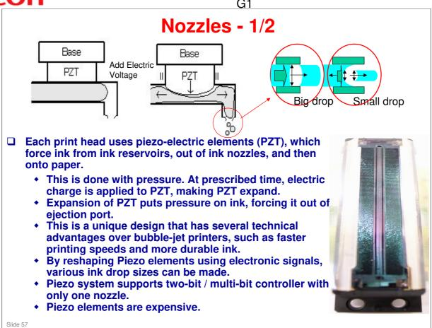
Note: View above is of head with it's surface cover removed.
