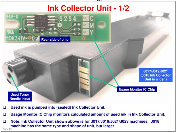
Note that the previous model Ink Collector Unit had a large opening for ink to fall into. New model is sealed – ink is pumped in.
