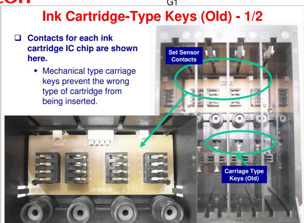
Note: These photos are from previous machine. Note that the mechanical keys are of a different shape from the new machine.
