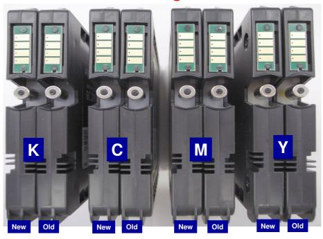
Different mechanical keys at end of new type cartridges safeguard against using wrong generation cartridges in machine.
