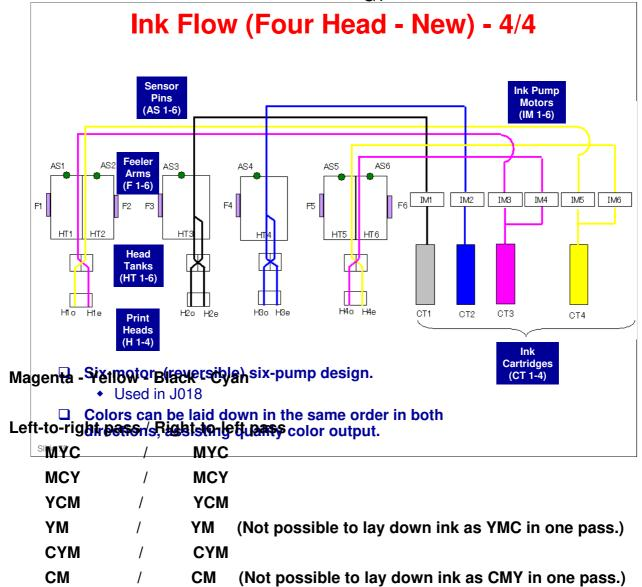
Colors can be laid down in the same order in both directions, assisting quality color output, but there are some color combinations that can not be laid down in one pass.
