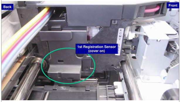
□ 1st registration sensor detects leading edge of every sheet, and also detects width of paper when carriage and sensor pass horizontally over vertical edge of paper as it feeds.
