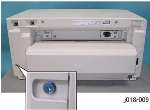
1. Remove the screw at the right rear corner (
