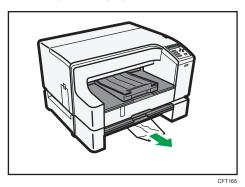
If you cannot remove the jammed paper or it is difficult to remove, the paper may be jammed inside the printer. See "Removing Paper Jammed around the Guide Board" or "Removing Paper Jammed in the Duplex Unit" and remove jammed paper from inside the printer.
