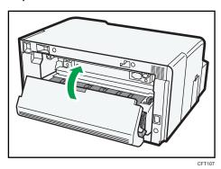
If the bypass tray is attached to the printer, switch the printer off and detach the bypass tray. Check that the duplex unit is correctly attached and the duplex unit cover is closed.
