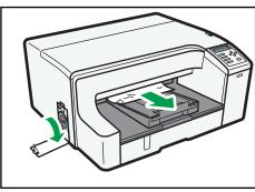
If turning the paper wheel does not remove the jammed paper, use the following procedure to remove it:
