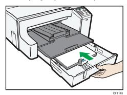
10. Pull out the output ramp extension.
