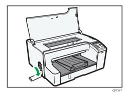
3. Remove the jammed paper through the top cover opening or back of the printer.
