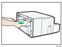
8. Attach the multi bypass tray until the lever for multi bypass tray attachment and detachment clicks.
