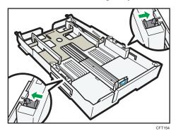
5. Pinch the catch of the paper guide on the right side, slide the paper guides to match the size of paper you want to load, and then push the end paper guide out until there is space between them.
