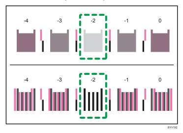
Combined two-color lines form squares, and depending on line overlapping, (white) spaces between the lines are painted and look darker. Sometimes the colors of the lines are identical.
