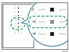
When horizontal lines beside the lightest gray square are broken, select the optimal adjustment value by referring to the lines broken in the opposite direction. When the "+2" square is the lightest gray square and the "+6" horizontal lines are broken in the opposite direction, the optimal adjustment value is between "+3" and "+5". After adjustment, check the adjustment result.
