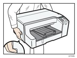
Grip the indented area at the base of the printer's sides, as shown. Lift and carry the printer slowly and carefully.
