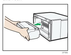
If using the GX e2600, attach the rear cover.
