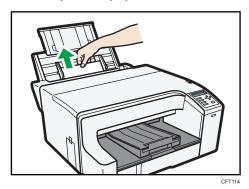
3. Load paper in the bypass tray with the side to be printed on facing up.
