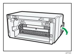
5. Turn the paper feed wheel to release paper from the feed belt.
