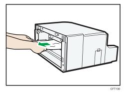
4. Without pressing the catches on its sides, push the duplex unit all the way in until it clicks into place.
