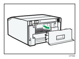
3. Unlock the guide board by moving the tabs on both sides toward the middle, and then open the guide board.
