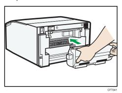
If the bypass tray has been detached, be sure to switch the power off before reattaching the tray.
