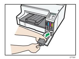
6. Slide the ink collector unit carefully into the printer, until you hear it click.
