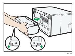
If using the GX e2600, remove the rear cover.
