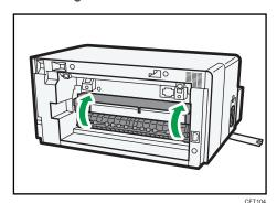
Push the PUSH area on both sides of the guide board until it firmly closes.
