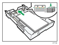
7. Squeeze the front end paper guide, and then slide it to meet the edge of the paper.
