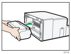
If the multi bypass tray has been detached, be sure to switch the power off before reattaching the tray.
