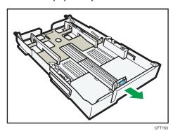
4. Slide both tabs to the original positions, and then lock the tray.
