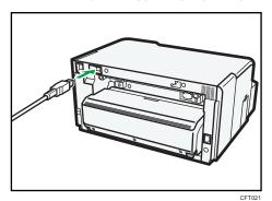
4. Insert the USB cable's rectangular (type A) plug firmly into the computer's USB slot.
