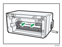
Before removing jammed paper from the back of the printer, remove the duplex unit.
