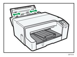
Press the lever on the side of the paper guide while moving the guide.
