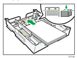
4. Squeeze the front end paper guide, and then slide it to meet the edge of the paper.
