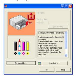
The illustration above indicates the cyan Print cartridge has completely run out.
