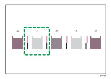
A vertical line of a square consists of two overlapping lines, so if the print head is not positioned properly, the line looks misaligned.
