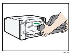
5. Connect the power cord, USB cable, or Ethernet cable.
