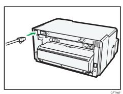
2. Connect the other end of the cable to the printer's network, such as to a hub.
