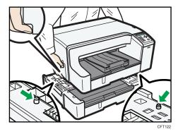
Grip the center area at the base of the printer's sides. Lift it slowly and do not strain your body.
