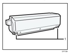
3. Remove the jammed paper from the rear of the printer.
