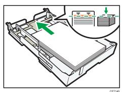
7. Squeeze the front end paper guide, and then slide it to meet the edge of the paper.
