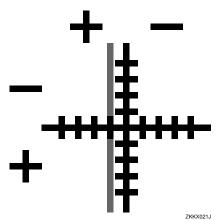
11. Fold the test pattern sheet in half widthwise, and then check the adjustment value for the [Feed Direction].
