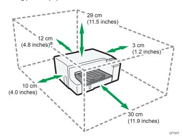
a. If you attach the bypass tray (option), provide additional clearance of 29 cm (11.5 inches).
