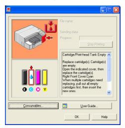
The illustration above indicates the cyan ink has completely run out.
