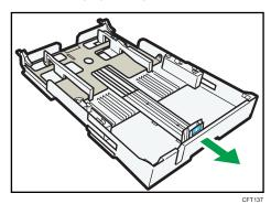
4. Slide both tabs to the original positions, and then lock the tray.
