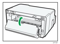
If the bypass tray has been detached, be sure to switch the power off before reattaching the tray. Printing starts.
