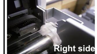
9. Clean the strip with alcohol by wiping the surface from right to left.
