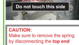
**CAUTION:** Make sure to remove the spring by disconnecting the top end (shown by the arrow in the photo).
