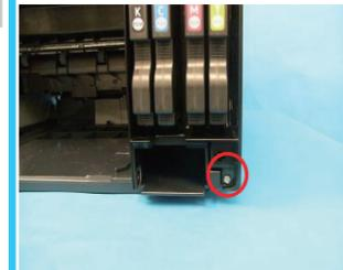
3. Release the tab on the front left corner of the machine.
