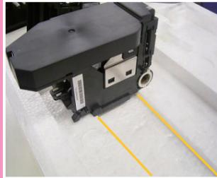
Removal of the carriage unit completed.
