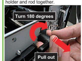
**CAUTION:** Make sure to secure the carriage unit in place with one hand while you remove the guide rod with the other hand.
