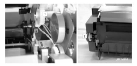
The main gear [1] of the vertical motor of the printer drives the duplex drive gear [2].
