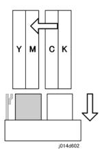
When the cleaning cycle starts, the maintenance unit is lowered by the rotation of the main shaft. The cams rotate away from the bottom of the unit.
