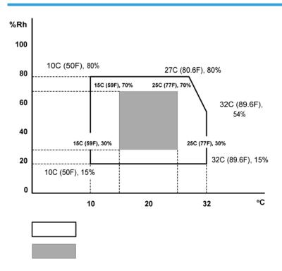
Set up the machine in a location that meets these minimum requirements:
