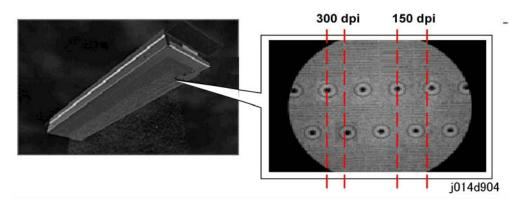
During 150 dpi printing only one line of nozzles eject ink as shown above. During 300 dpi printing the nozzle ports (alternately offset as shown above) of both lines eject ink.
