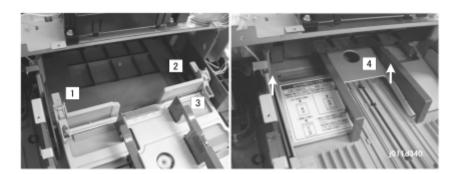
The arms [1] and [2] on both sides of the cassette [3] (guided by rails slanting upward) raise the bottom plate [4] when the paper cassette is pushed into the printer. This raises the paper in the cassette to the correct height for paper feed.
