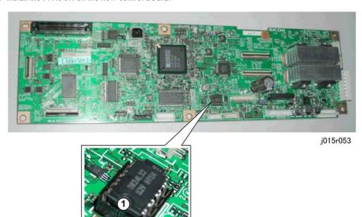
3. Attach the new NVRAM so the curvature of the white line on the board ① matches the curvature of the indentation ② on the NVRAM chip.
