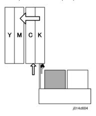
Next, the maintenance unit lowers, and another cam raises the wiper. At the same time the carriage moves the print heads left far enough so the vacuumed print head brushes past the wiper. The wiper cleans the ink from the print head.
