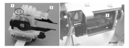
A pair of vertical sensor pins [1] is provided for each tank. These pins detect changes in the voltage differential on the surface of the ink inside the print head tank to detect the presence of air. When these terminals detect air in the tank, air escapes through the air release valve [2] opened by the air release solenoid [3]. This allows more ink to enter the tank.
