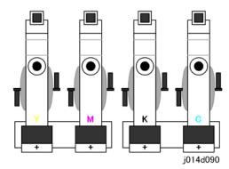
The illustration above shows the arrangement of the print heads and print head tanks.
