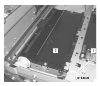
This printer uses the BT (Belt Transfer) system to transport paper through the paper path.
