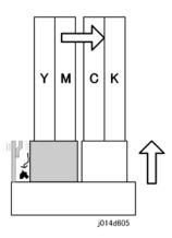
Next, the carriage moves the print heads back to the home position. The maintenance unit caps the print heads. A cam on the main shaft below vibrates the small scraper. This removes the ink bolus from the wall of the trap and sends it to the ink collector unit.
