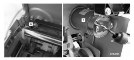
The picture above shows the horizontal driver gear [6] of the horizontal drive motor [7] mounted on the left rear corner of the printer behind the duplex unit.
