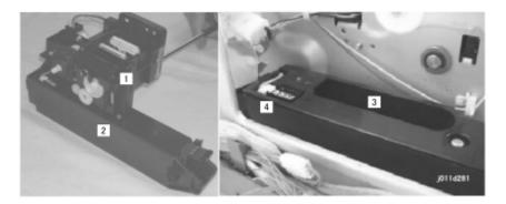
Inside the printer, the maintenance unit [1] sits on top of the ink collector unit [2].
