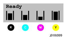
The printer shows a 6-level dynamic display that keeps the operator informed about the status of the ink levels in the tanks. The example below for Black (K)shows the progression in the display from full on the left to completely empty on the right.
