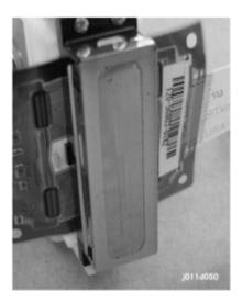
The wide print head increases the width of the band printed with one pass. This lets the machine print faster.
