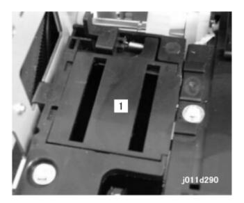
During a long print job, the machine flushes all the nozzles with a very small amount of ink at about 15 second intervals. The ink flushed from the nozzles goes through the slots of the flushing gate [1] into a sump below. This keeps the nozzles clear and in good working condition.
