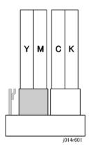
Cleaning starts with the carrier and print heads capped and resting on top of the maintenance unit as shown above.
