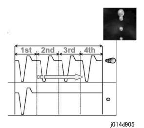
Four dots are required to form a large drop but only one is sufficient for a small drop. The four dots for a large drop are ejected very quickly as they form one dot before they reach the surface of the paper. The 4th dot in this case is ejected extremely fast under high pressure (1 Mega Pascal).
