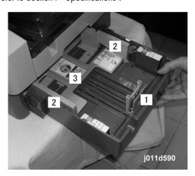
You can adjust and lock the end fence [1] and two side fences [2] to a variety of standard paper sizes.
