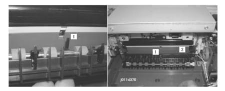
The feeler [1] is pushed down by every sheet of paper that arrives and then pops up again when the trailing edge of the sheet passes over the feeler. When the paper presses down the feeler, this turns on the trailing edge sensor [2]. The length of time the trailing edge sensor remains on is used to measure the length of the paper for printing control.
