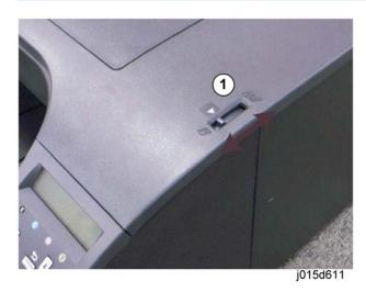
Move the envelope selector ① to adjust size of the gap between the print heads and the surface of the paper.
