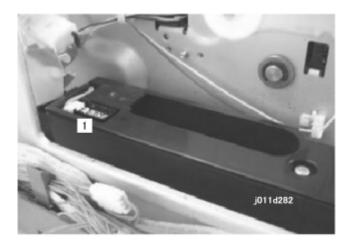
The ink collector ink level sensor [1] is a "smart" reflective photosensor.
