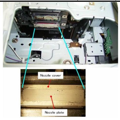
4. Clean each side of the nozzle twice with a slightly damp cloth. **Important:** Move the cloth back and forth along the surface.
