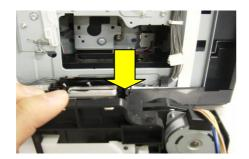
2. Turn the motor shaft manually in the direction of the arrow until the motor lock is released.
