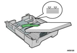
5. Squeeze the front end paper guide, and then slide it to meet the edge of the paper.
