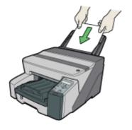
Printing cannot start until the machine finishes cleaning its head. Load the paper in the bypass tray when cleaning finishes.
