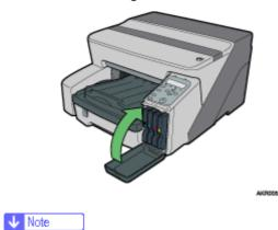
• If the error persists, take the Print cartridge out once, and then install it again. The procedure above should be performed only once.
