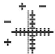
10. Fold the test pattern sheet in half widthwise, and then check the adjustment value for the [Feed Direction]
