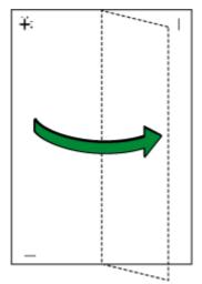
10. The optimal adjustment value is the difference between the single vertical line and the cross's vertical line that you can see when the folded paper is held up to light. When the difference is one calibration mark in the "+" direction, the optimal adjustment value for the [Printing direction:] is "+1.0".
