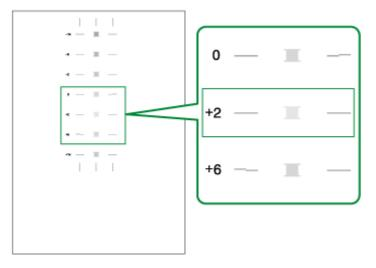
The optimal adjustment value is the number that appears on the left of the lightest gray square with straight horizontal lines on both sides. When this number is "+2", the optimal adjustment value is "+2".
