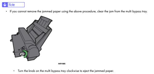
• If this does not eject the paper, turn the knob one-turn counterclockwise, and then turn it clockwise. This will eject the paper.
