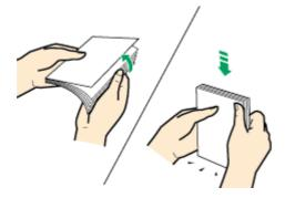
• Before loading envelopes, make sure their edges are sharply creased by rubbing the edges with a pen or similar object.
