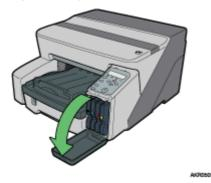
2. Push in the cartridge using the PUSH area.
