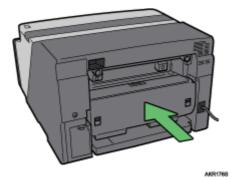
7. Lock the lever for attaching the duplex unit.
