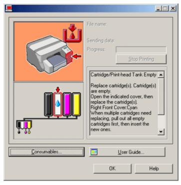
In this illustration, the cyan ink has completely run out.
