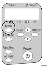
Press [▲] or [▼] to scroll to "Counter" on the display, and then press the [#Enter] key.
