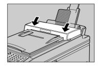
Fan the stack of originals. Never try to place more than 10 sheets of plain paper onto the ADF.
