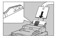
Squeeze the tray guide and slide it against the edge of the stack.
