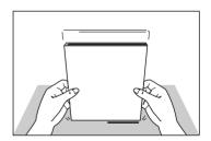
Place the stack of originals face down on the ADF and slide the document guide against the side of the stack.
