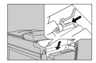
To install the upper paper tray, press down on both sides of the tray, making sure that it is inserted as far as it will go.
