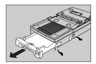
After removing all tapes and cardboard from inside of the paper tray, insert the tray back into the machine until it locks into place. Locate the paper feed unit where you plan to use the machine.
