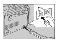
Connect the other end of the telephone handset cable to your telephone.
