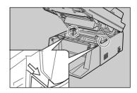
Make sure the plastic pins (marked with "\*" in the illustration next to step 3) on either side of the starter toner cassette slide along the guides inside the machine.
