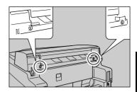
Insert one end of the document output tray into the slot provided. Then gently bend the tray so the other end fits into the second slot.
