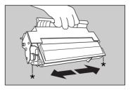
Look inside the machine and note the locations of the arrows that indicate the toner cassette guides on either side.
