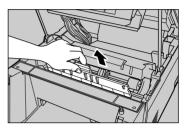
Grasp the new cleaning pad by the green handle and insert it into place.
