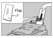
• Envelope flaps should be securely folded down, so the envelope is "closed". This is especially important when printing on envelopes with adhesive on the flaps because heat generated during the printing process can cause the adhesive to melt and get on rollers.
