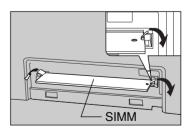
Carefully lift out the currently installed SIMM board.
