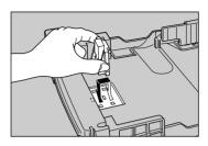
Squeezing in on both sides of the side guide, slide it to the correct position for the desired paper size.
