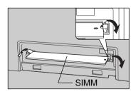
Carefully lift out the SIMM board currently installed on your printer.
