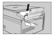
After setting the paper into the tray, raise the small panel until it snaps securely into place.
