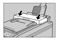
Fan the stack of originals. Never try to place more than 10 sheets of plain paper onto the ADF.
