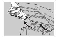
Pressing down on the paper release lever (blue) on the right side, pull out the misfed paper.
