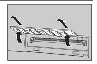
Angle the new SIMM board as shown in the illustration, and insert it down into the slot. Gently rock it back and forth until you hear it snap into place.
