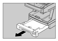
Press down on the metal plate in the bottom of the paper tray until the plate locks into place with a "click".
