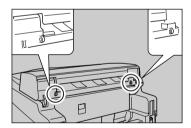
Insert the pin at one side of the tray by gently bending the document tray until it fits in the insert hole.
