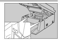
Make sure the plastic pins (marked with "\*" in the illustration next to step above) on either side of the toner cassette slide along the guides inside the machine.
