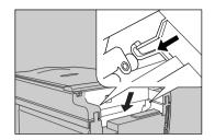
To install the upper paper tray, press down on both sides of the tray, making sure that it is inserted as far as it will go.
