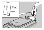
• Envelope flaps should be securely folded down, so the envelope is "closed". This is especially important when printing on envelopes with adhesive on the flaps, because heat generated during the printing process can cause the adhesive to melt and get on rollers.
