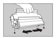
Look inside the machine and note the locations of the arrows that indicate the toner cassette guides on either side.
