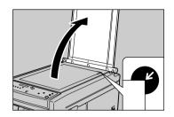
Open to the page you want to copy and lay the page face down on the exposure glass. Be sure to align one of the corners of the page with the arrow mark on the scale.
