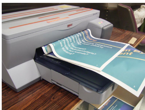
Fig.3: Abnormal condition (Paper jam)
