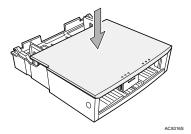
7 Align the connecting parts of the printer and paper feed unit, and then place the printer on top of the paper feed unit.
