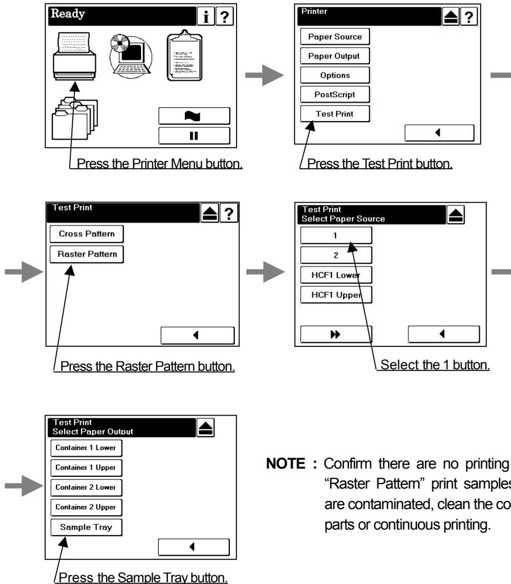
**NOTE :** Confirm there are no printing contamination on "Raster Pattern" print samples. If print samples are contaminated, clean the contaminated parts or continuous printing.
