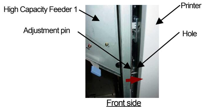
**CAUTION** When the height of a adjustment pin does not suit, please place the spacer of two sheets, and let slide and connect it with the bottom of a jack. (Ref4.8)
