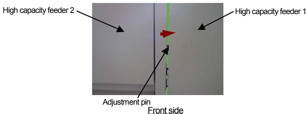
**CAUTION** When the height of a adjustment pin does not suit, please place the spacer of two sheets, and let slide and connect it with the bottom of a jack. (Ref4.8)
