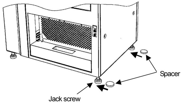
**CAUTION** When the height of a adjustment pin does not suit, please place the spacer of two sheets, and let slide and connect it with the bottom of a jack.
