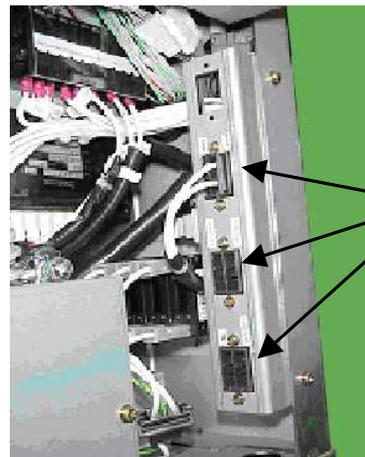
Measurement point of AC voltage
