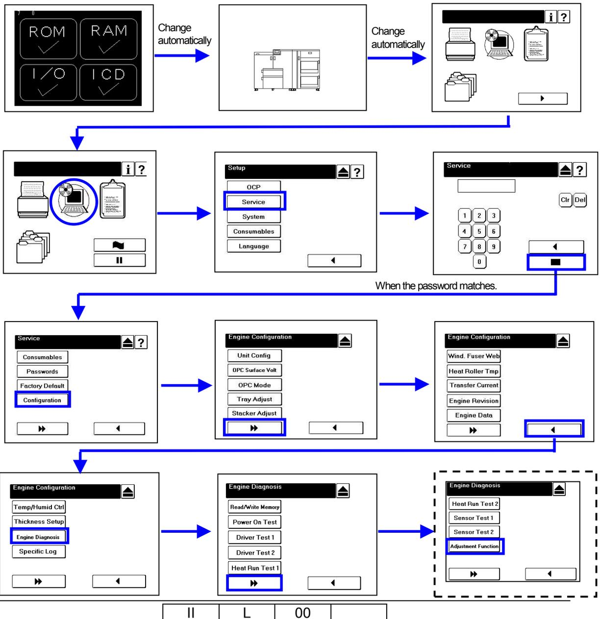
Access method to the Adjustment function on the OCP is shown below.
