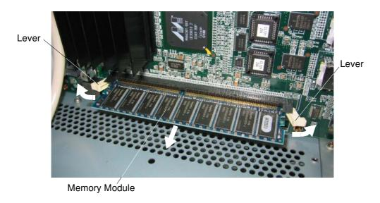
Figure 5-8. Releasing a DIMM
