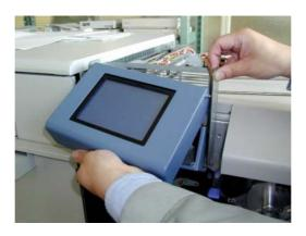
Figure 5-15. Removing the Operator Control Panel (7)
