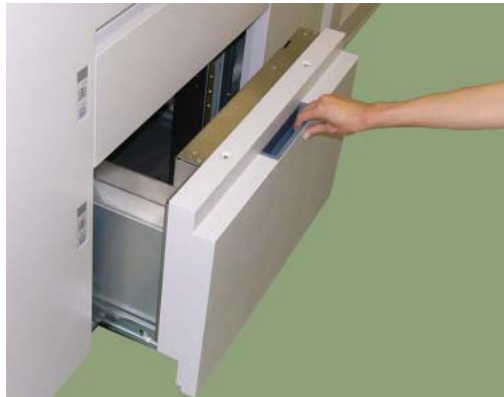
Figure 3-6. Loading Paper in Tray (2)
