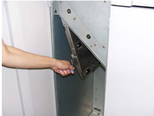
Figure 4-45. Clearing Paper from the Regist Cover (4)
