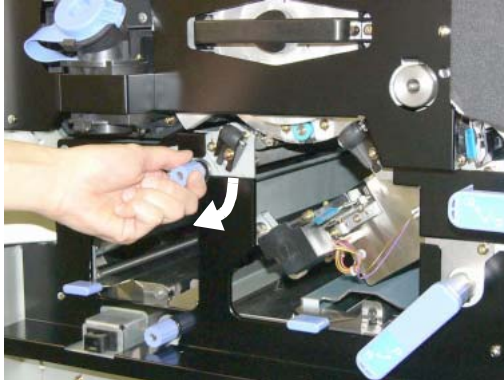
Figure 4-58. Clearing Paper from the Paper Feed Area (4)
