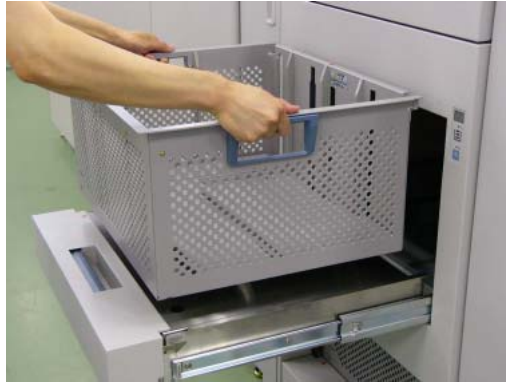
Figure 4-92. Clearing Paper from the Container Stacker (10)
