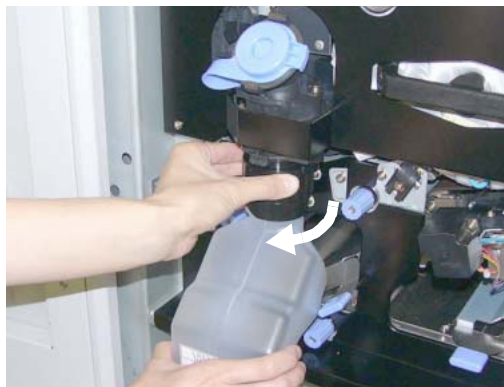
Figure 4-17. Replacing the Developer Mix (7)
