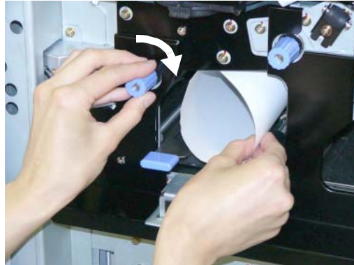
Figure 4-54. Clearing Paper from the Regist Station Area (4)
