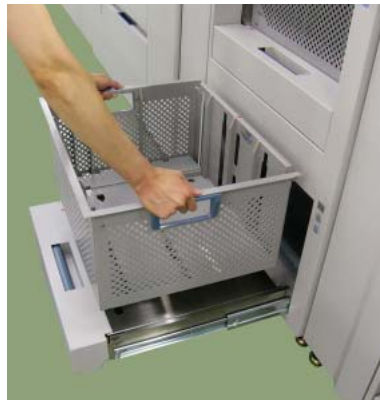
Figure 4-95. Clearing Paper from the Container Stacker (13)
