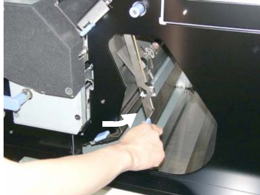
Figure 4-70. Clearing Paper from the Paper Feed Area (16)
