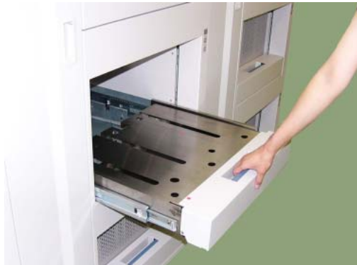
Figure 3-35. Set the Basket into the Stacker (2)
