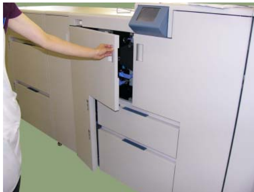
Figure 4-47. Clearing Paper from the Input Station Area (2)
