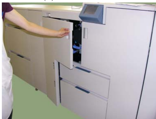
Figure 4-52. Clearing Paper from the Regist Station Area (2)
