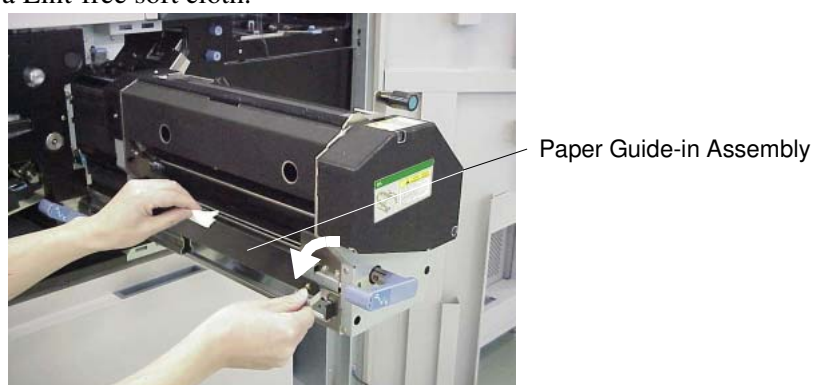
Figure 4-122. Cleaning the paper guide of the Fuser Unit (3)
