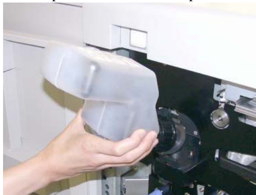
Figure 4-20. Replacing the Developer Mix (10)
