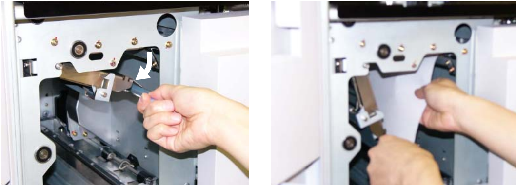
Figure 4-50. Clearing Paper from the Input Station Area (5)
