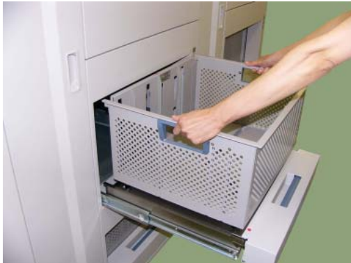
Figure 3-36. Set the Basket into the Stacker (3)
