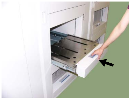
Figure 4-90. Clearing Paper from the Container Stacker (8)
