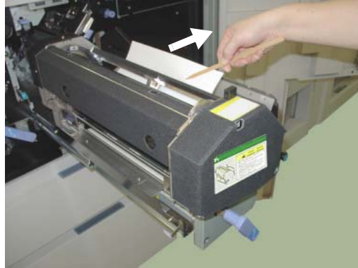
Figure 4-66. Clearing Paper from the Paper Feed Area (12)
