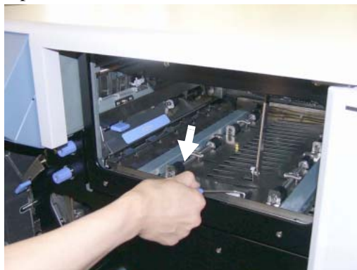
Figure 4-82. Clearing Paper from the Paper Feed Area (28)
