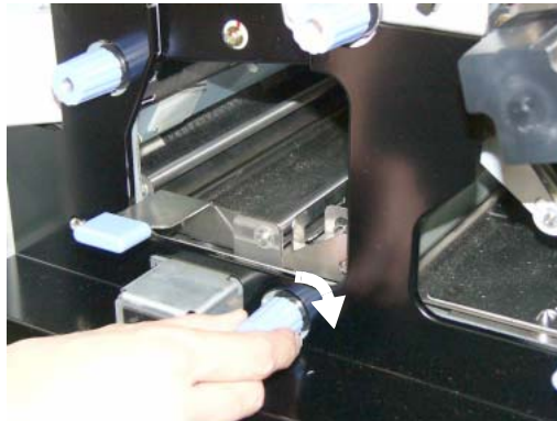
Figure 4-74. Clearing Paper from the Paper Feed Area (20)
