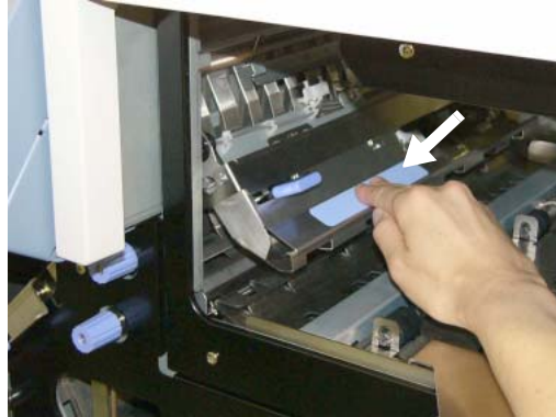
Figure 4-79. Clearing Paper from the Paper Feed Area (25)
