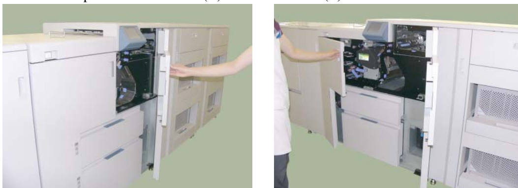
Figure 4-56. Clearing Paper from the Paper Feed Area (2)
