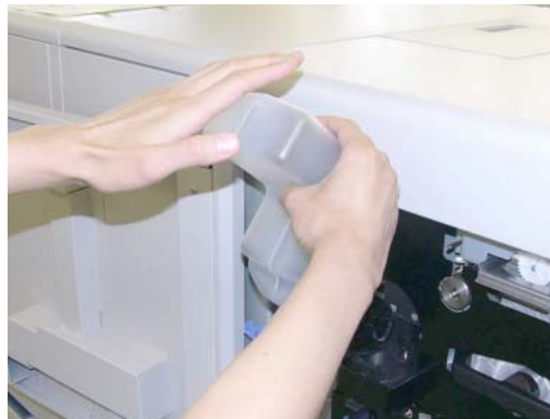
Figure 4-24. Replacing the Developer Mix (14)
