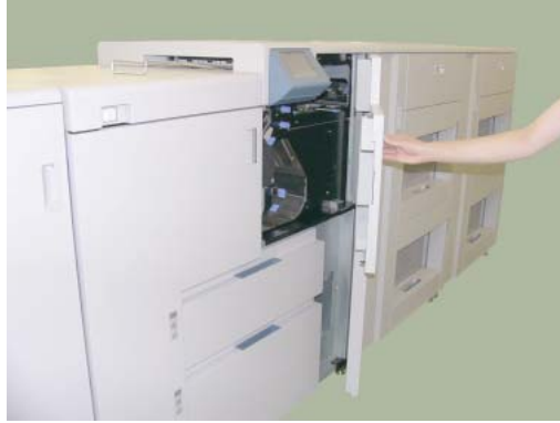
Figure 4-8. Replacing the Toner Bag (1)
