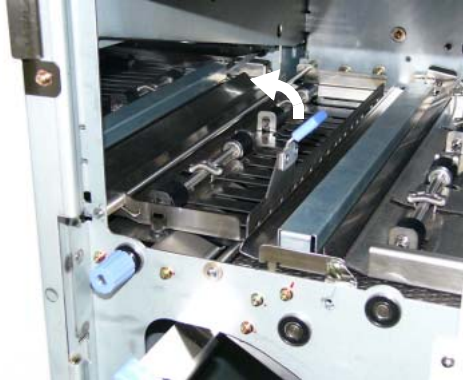
Figure 4-86. Clearing Paper from the Container Stacker (4)
