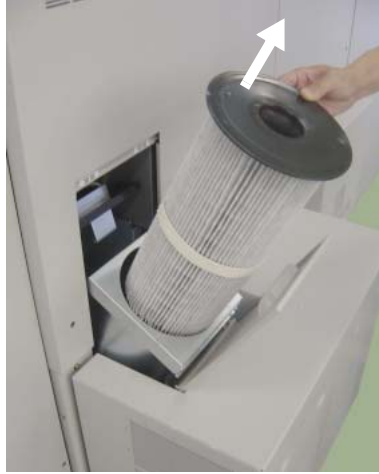
Figure 4-36. Replacing the Fine Filter (3)
