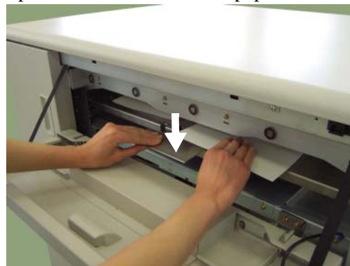
Figure 4-105. Clearing Paper from the High Capacity Feeder (8)
