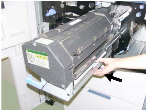
Figure 4-31. Replacing the Fuser Cleaning Web (5)
