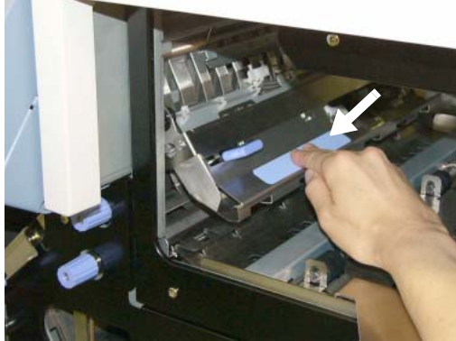
Figure 4-119. Cleaning the Inverter Valve Piece (4)
