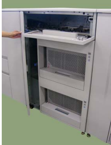
Figure 4-96. Clearing Paper from the Container Stacker (14)
