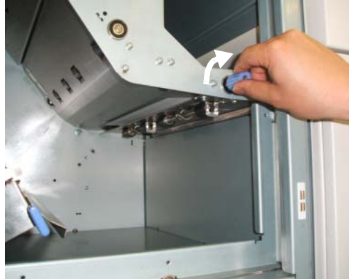
Figure 4-109. Clearing Paper from the Transit Pass Unit Type 156 (4)
