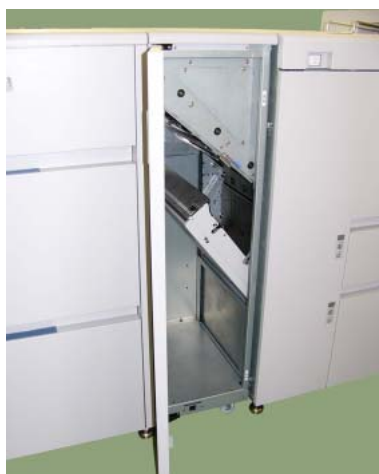
Figure 4-43. Clearing Paper from the Regist Cover (2)
