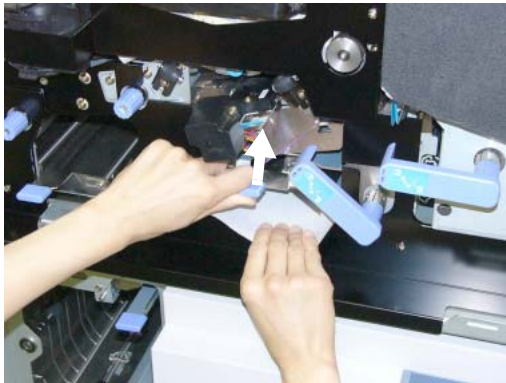
Figure 4-75. Clearing Paper from the Paper Feed Area (21)
