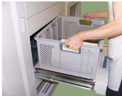
Figure 3-40. Removing paper from the Stacker (4)
