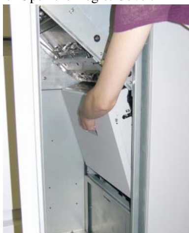
Figure 4-43. Clearing Paper from the Regist Cover (2)
