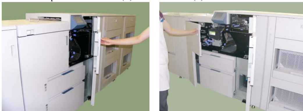
Figure 4-125. Cleaning the paper guide of the Discharger Unit (1)
