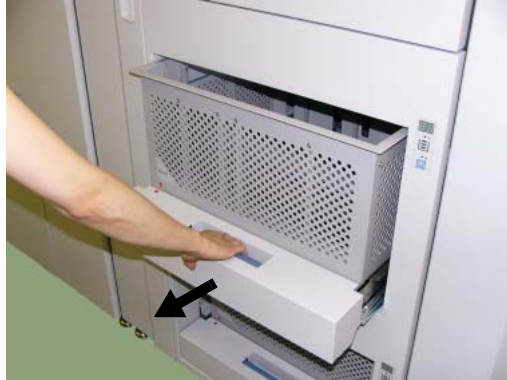
Figure 4-89. Clearing Paper from the Container Stacker (7)
