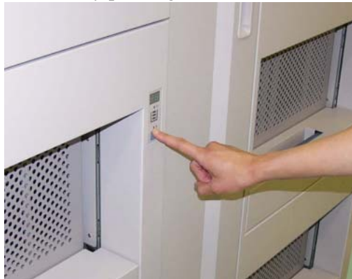
Figure 3-38. Removing Paper from the Stacker (2)
