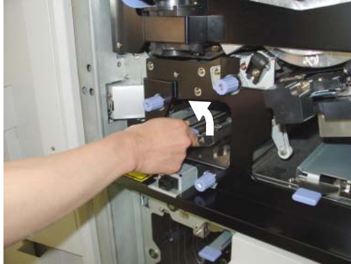
Figure 4-76. Clearing Paper from the Paper Feed Area (22)
