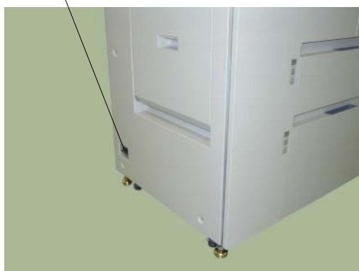
Figure 1-3. Powering On the Printer
