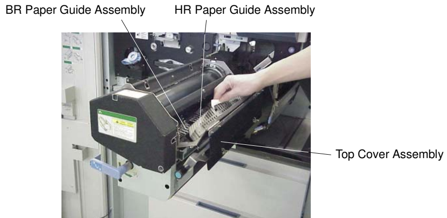
Figure 4-123. Cleaning the paper guide of the Fuser Unit (4)
