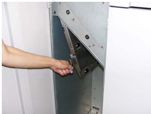
Figure 4-100. Clearing Paper from the High Capacity Feeder (3)
