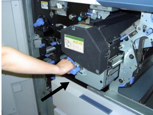
Figure 4-128. Cleaning the paper guide of the Discharger Unit (4)
