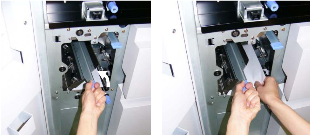
Figure 4-49. Clearing Paper from the Input Station Area (4)
