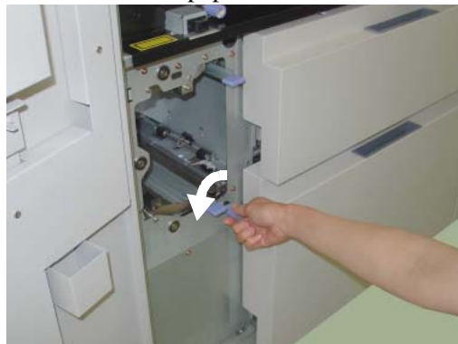
Figure 4-48. Clearing Paper from the Input Station Area (3)
