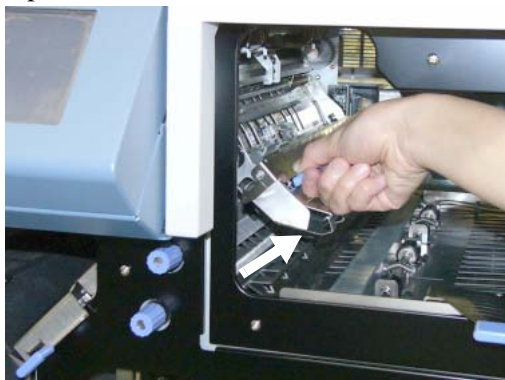
Figure 4-117. Cleaning the Inverter Valve Piece (2)
