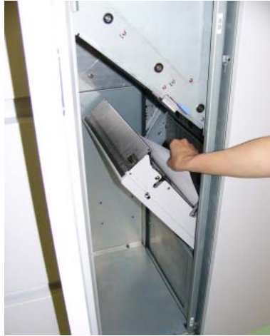
Figure 4-44. Clearing Paper from the Regist Cover (3)
