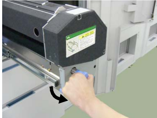
Figure 4-63. Clearing Paper from the Paper Feed Area (9)
