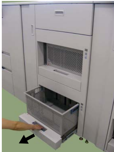
Figure 4-93. Clearing Paper from the Container Stacker (11)
