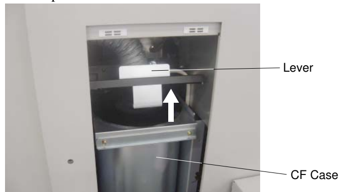
Figure 4-35. Replacing the Fine Filter (2)
