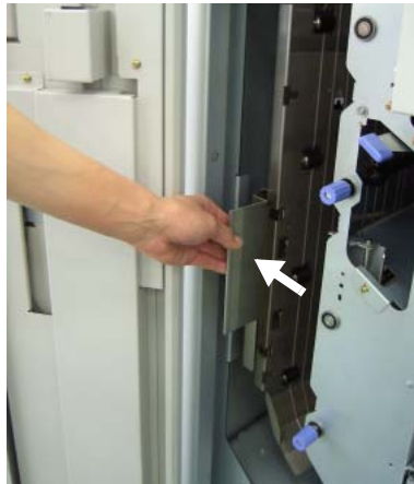
Figure 4-102. Clearing Paper from the High Capacity Feeder (5)
