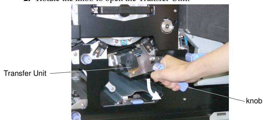
Figure 4-57. Clearing Paper from the Paper Feed Area (3)
