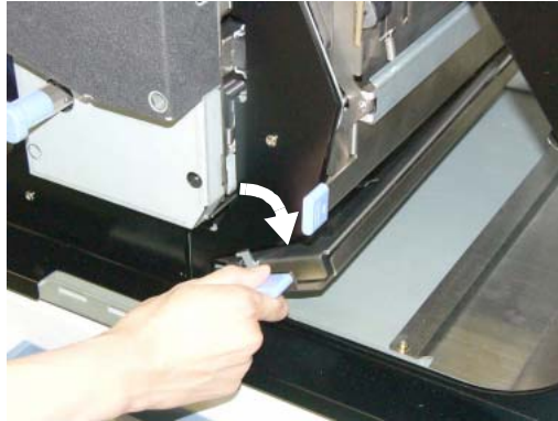
Figure 4-73. Clearing Paper from the Paper Feed Area (19)
