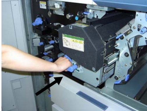
Figure 4-32. Replacing the Fuser Cleaning Web (6)
