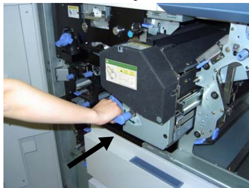
Figure 4-124. Cleaning the paper guide of the Fuser Unit (5)
