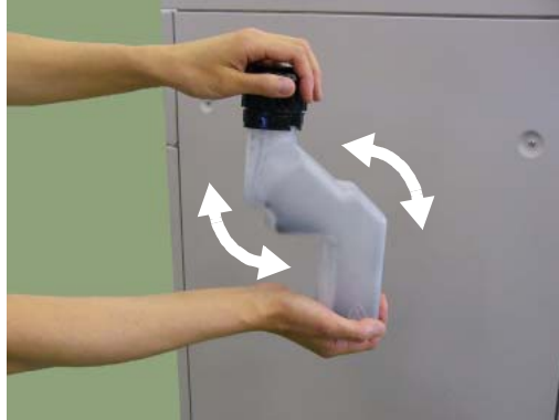
Figure 4-18. Replacing the Developer Mix (8)
