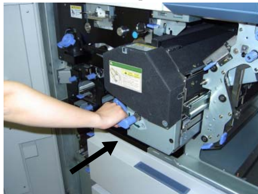
Figure 4-69. Clearing Paper from the Paper Feed Area (15)
