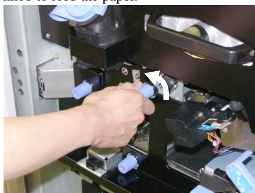
Figure 4-53. Clearing Paper from the Regist Station Area (3)
