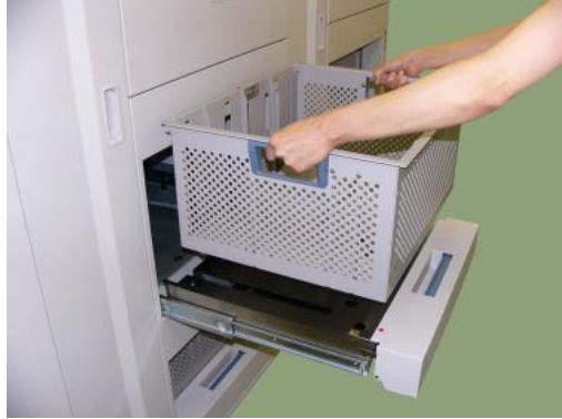
Figure 4-111. Cleaning the Container Baskets (1)
