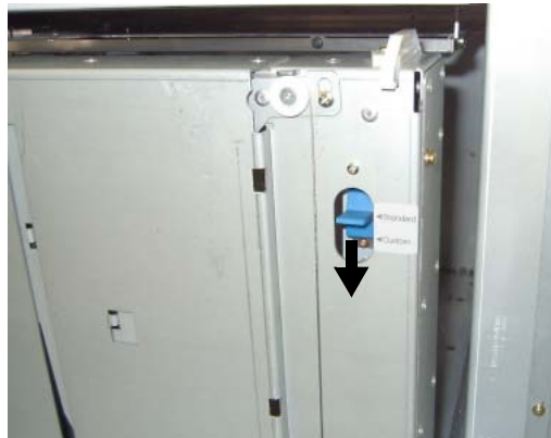
Figure 3-12. Setting the Non-Standard Paper Size(1)
