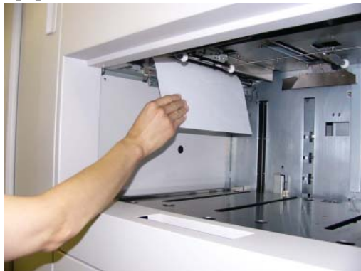
Figure 4-91. Clearing Paper from the Container Stacker (9)
