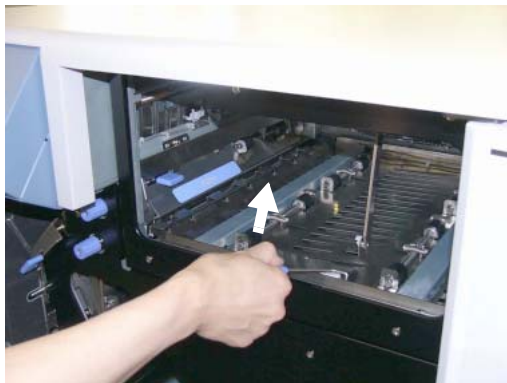
Figure 4-80. Clearing Paper from the Paper Feed Area (26)
