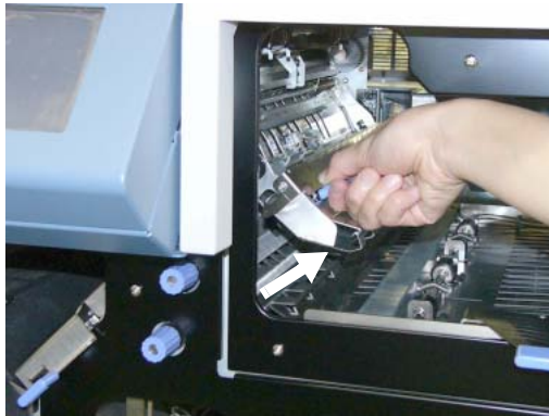
Figure 4-77. Clearing Paper from the Paper Feed Area (23)
