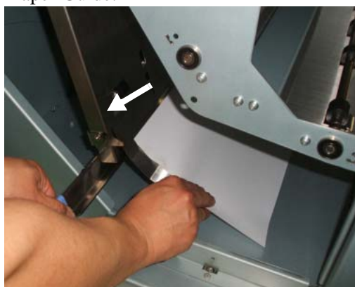
Figure 4-108. Clearing Paper from the Transit Pass Unit Type 156 (3)
