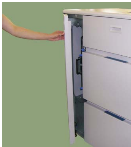
Figure 4-99. Clearing Paper from the High Capacity Feeder (2)
