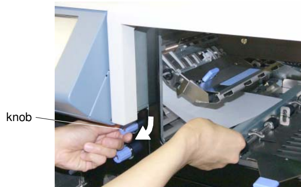
Figure 4-78. Clearing Paper from the Paper Feed Area (24)
