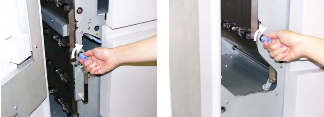
Figure 4-101. Clearing Paper from the High Capacity Feeder (4)
