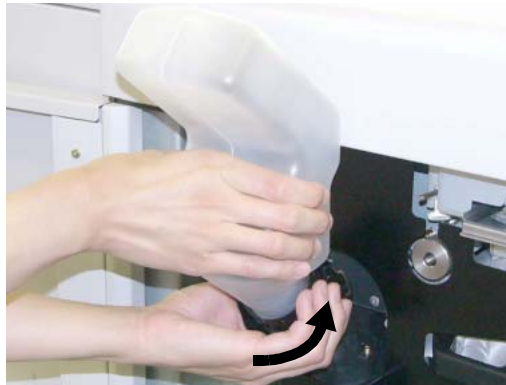
Figure 4-26. Replacing the Developer Mix (16)
