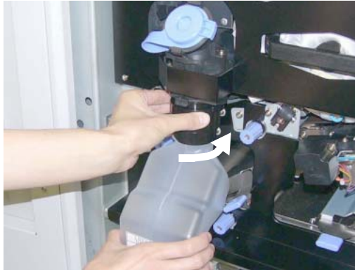
Figure 4-13. Replacing the Developer Mix (3)
