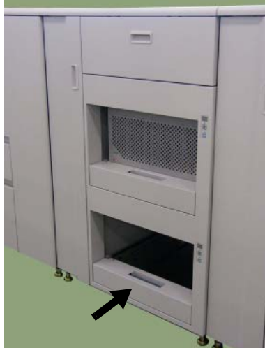
Figure 4-94. Clearing Paper from the Container Stacker (12)
