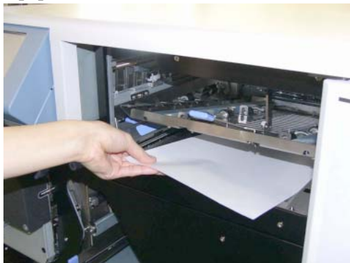
Figure 4-81. Clearing Paper from the Paper Feed Area (27)
