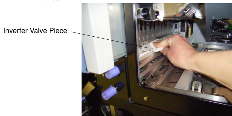
Figure 4-118. Cleaning the Inverter Valve Piece (3)
