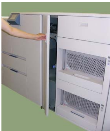
Figure 4-84. Clearing Paper from the Container Stacker (2)
