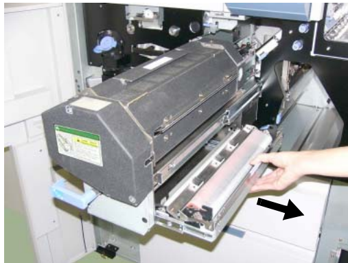
Figure 4-64. Clearing Paper from the Paper Feed Area (10)
