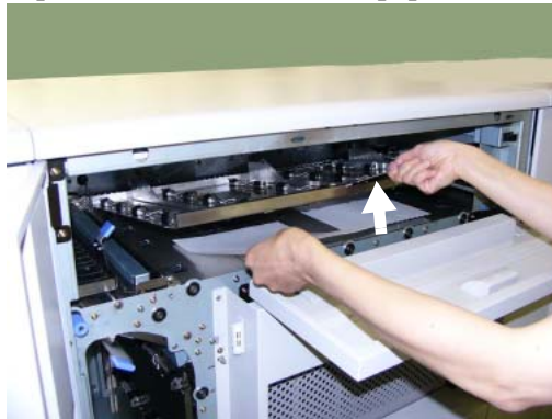
Figure 4-97. Clearing Paper from the Container Stacker (15)
