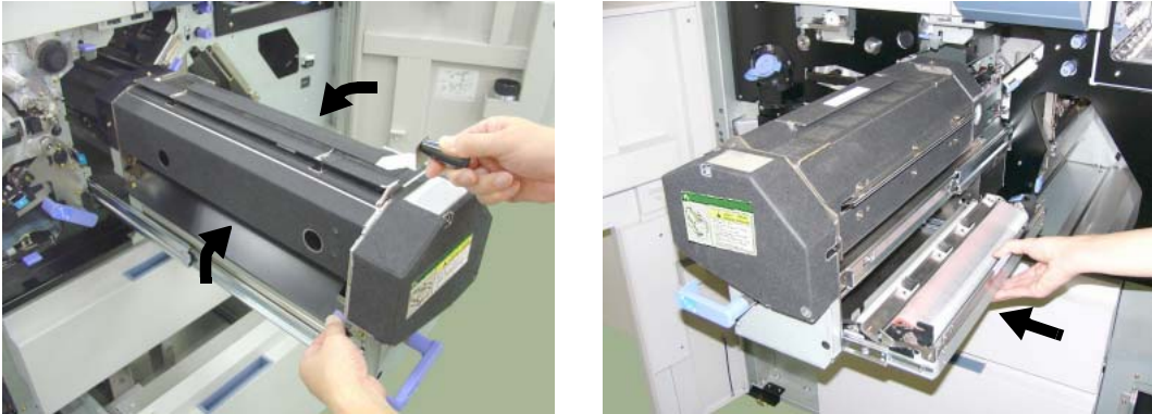
Figure 4-67. Clearing Paper from the Paper Feed Area (13)
