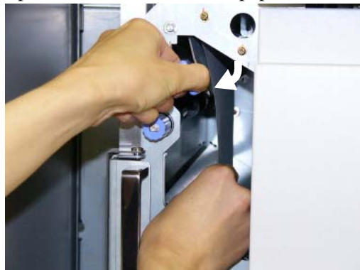
Figure 4-103. Clearing Paper from the High Capacity Feeder (6)
