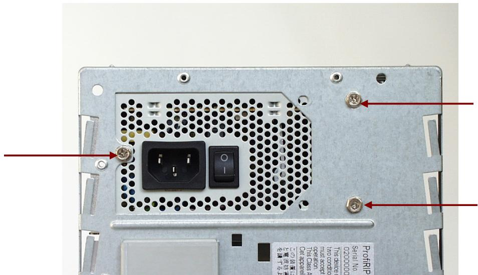
Hold the power supply in your hand when removing the screws, otherwise it may drop down and damage other components.
