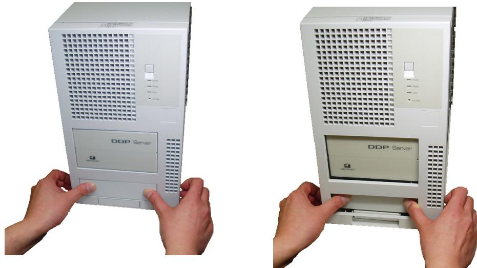
When the front cover is closed, push it to the chassis before it can be pushed into the hinges.
