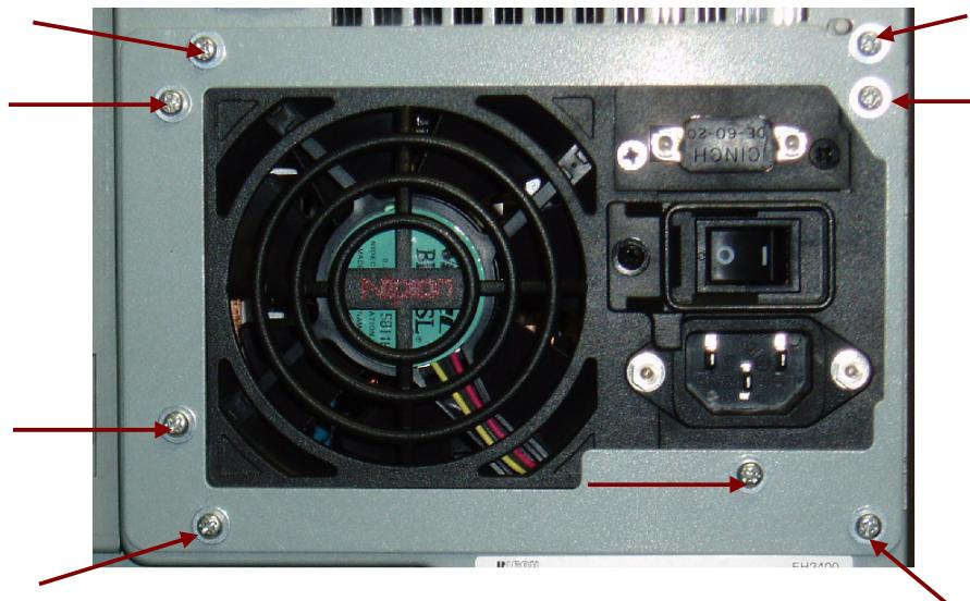
Hold the power supply in your hand when removing the screws, otherwise it may drop down and damage other components.
