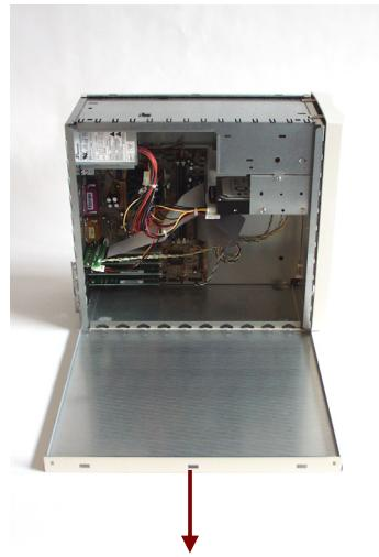
Each side cover must be in a 90° position to the chassis before it can be pushed into the hinges of the pivot fastener for closing. Do not apply force when attempting to close the cover. The side cover closes easily once the hinges are in the correct position.
