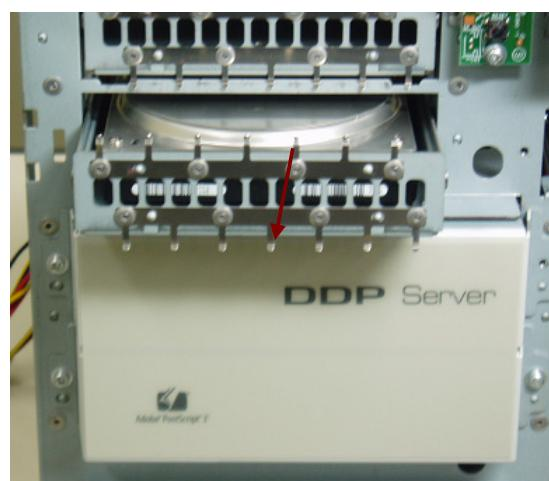
Then remove 4 screws fixing HDD on the tray.
