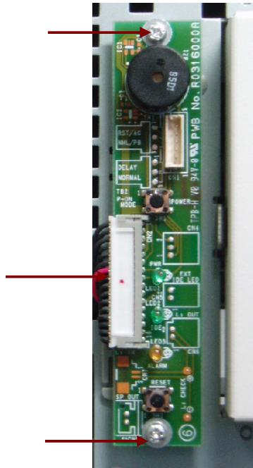
Make sure to reconnect the cables correctly after fixing the switch panel by 2 screws when installing the switch panel. Switch cable is polarized and cannot be inserted in wrong orientation.
