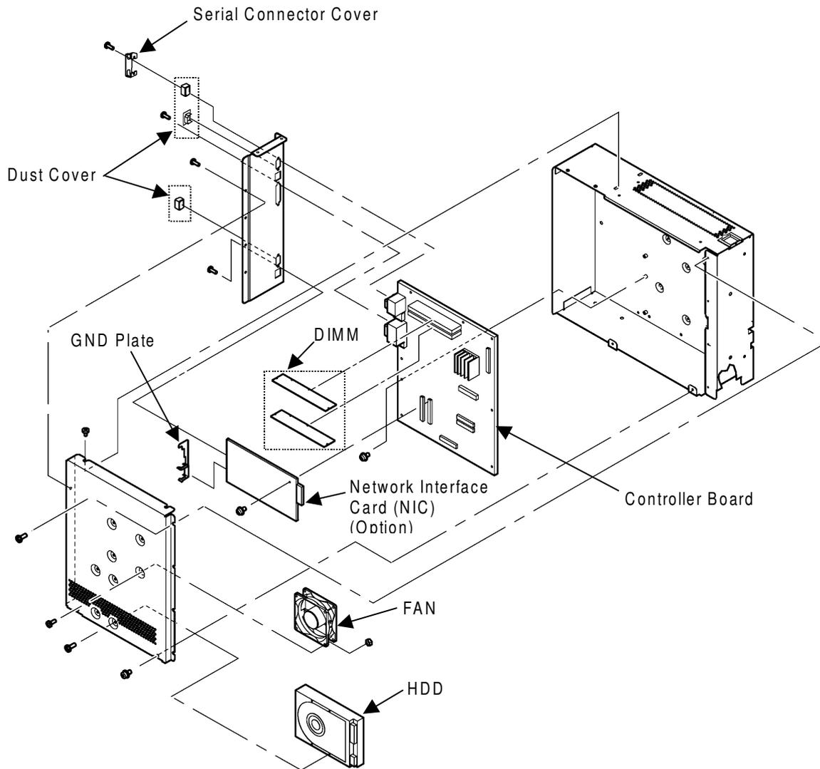
**Figure 4-7. Controller Assembly**
