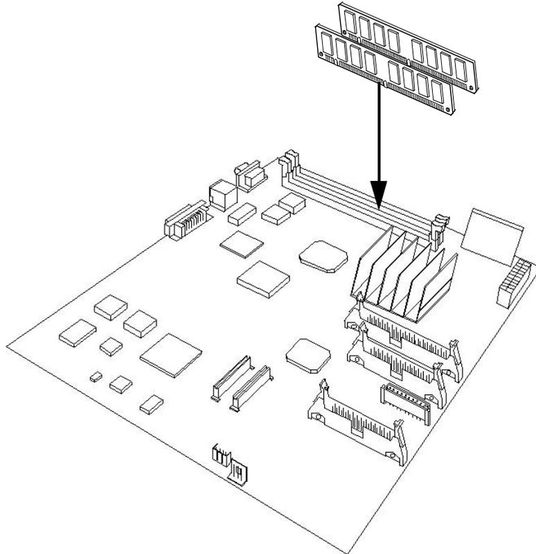
**Figure 4-8. DIMM Location on the Controller Board**
