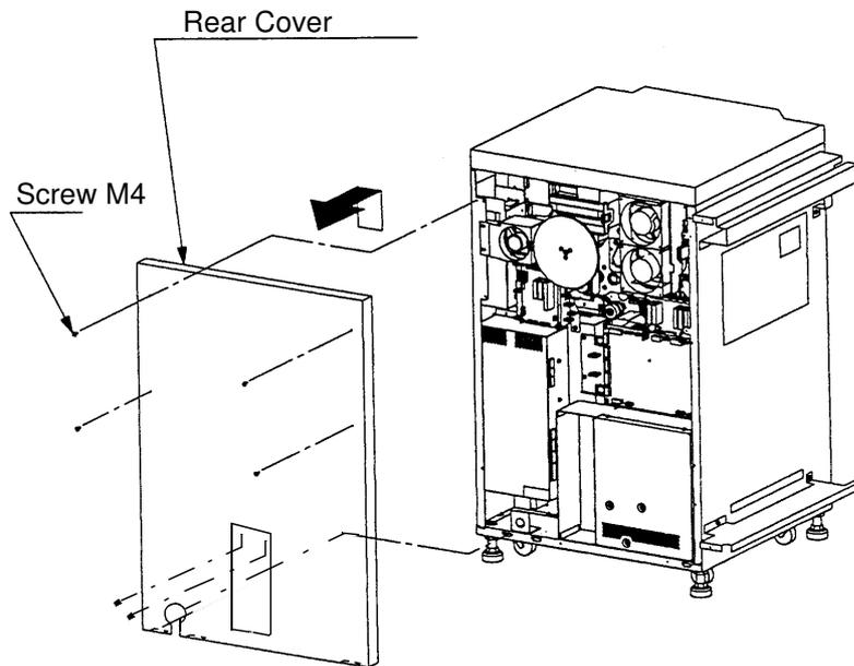
**Figure 4-2. Accessing the Controller Assembly**
