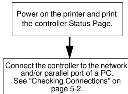
**Figure 4-4. Controller Connection Verification Steps**
