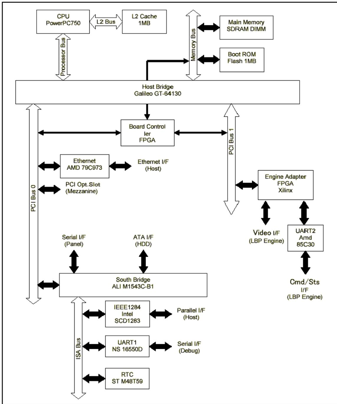
Figure 2-2. Controller Functional Diagram
