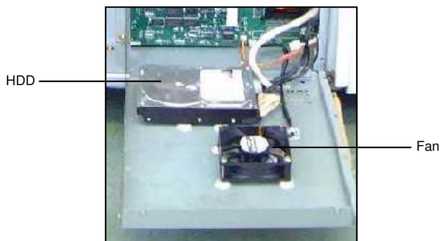
**Figure 4-10. Hard Disk Drive and Fan**
