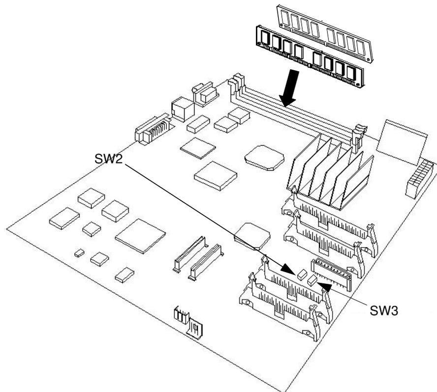
**Figure 5-7. DIMM Location on the Controller Board**
