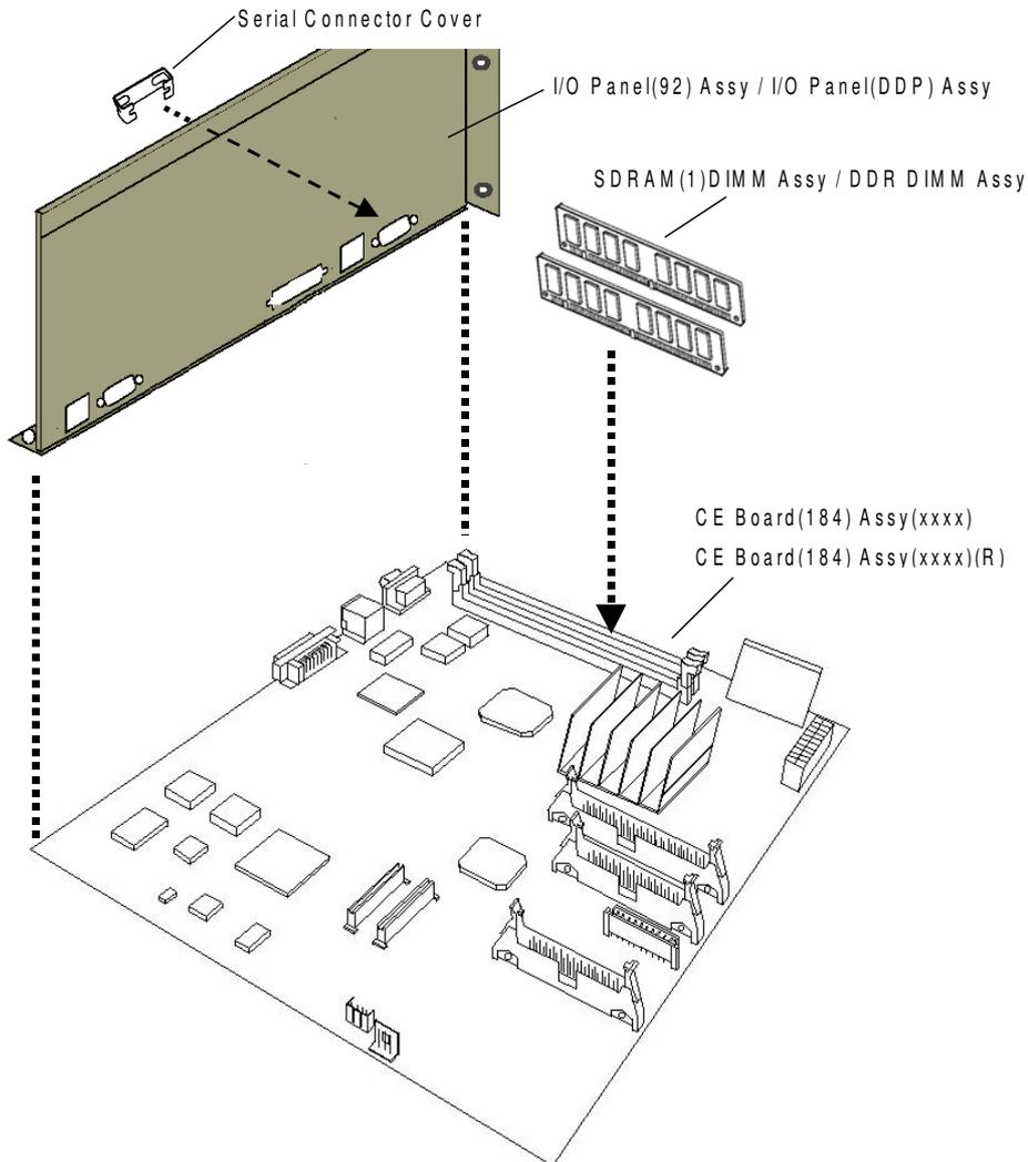
**Figure 5-1. Controller Assembly and Parts**
