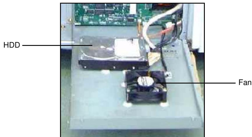
**Figure 5-9. Hard Disk Drive and Fan**
