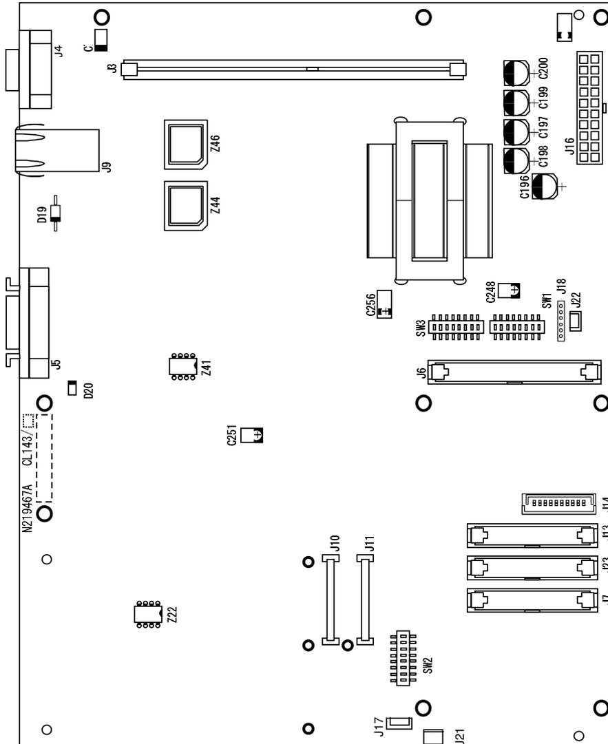
**Figure 5-5-1. Controller Board Layout (CL143/CL144)**
