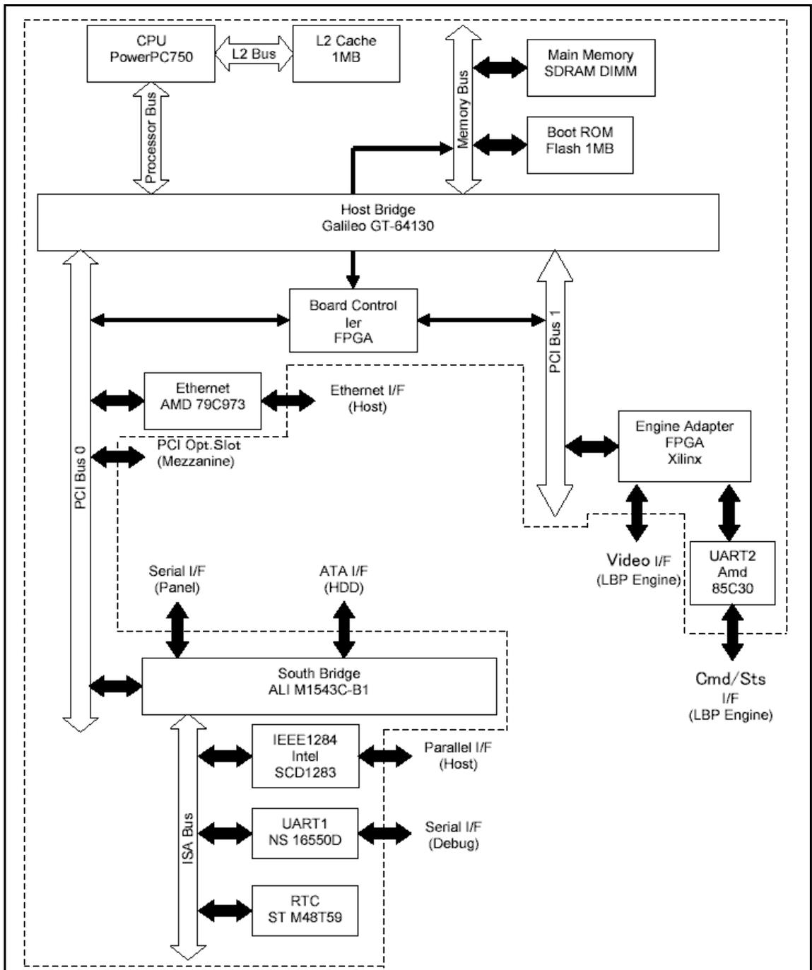
Figure 2-2. Controller Functional Diagram (CL106/CL107)
