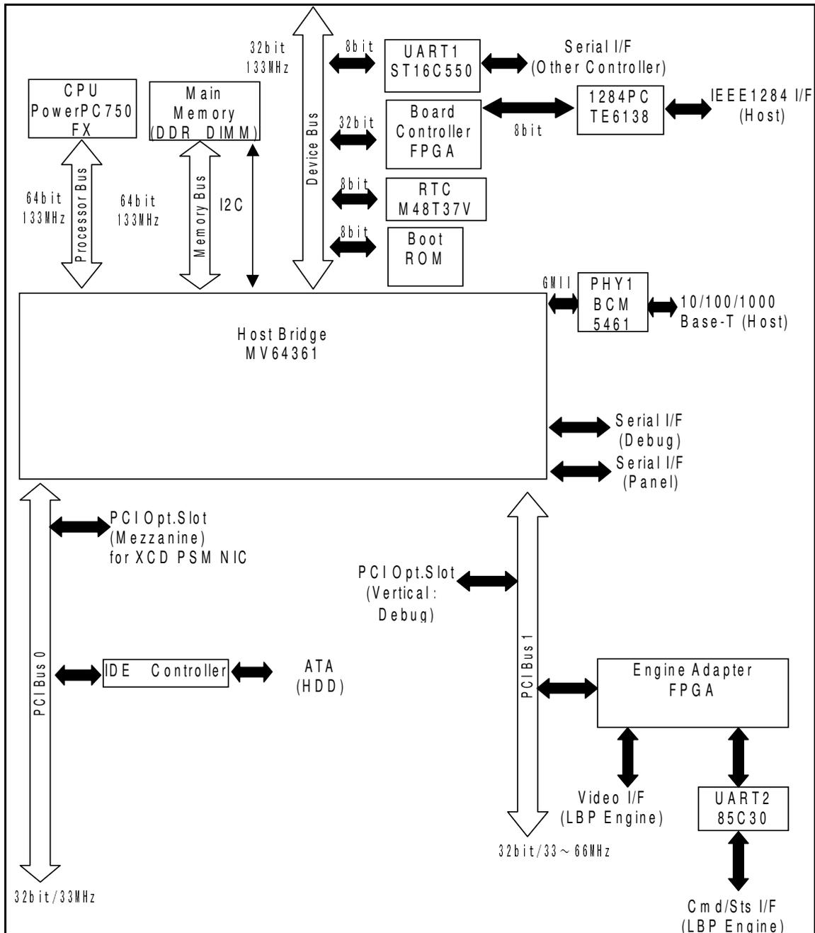
Figure 2-3. Controller Functional Diagram (CL143/CL144)
