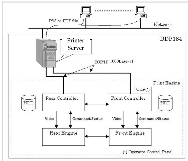
Figure 2-1. Controller Printing System
