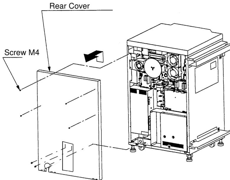
**Figure 5-2. Accessing the Controller Assembly**
