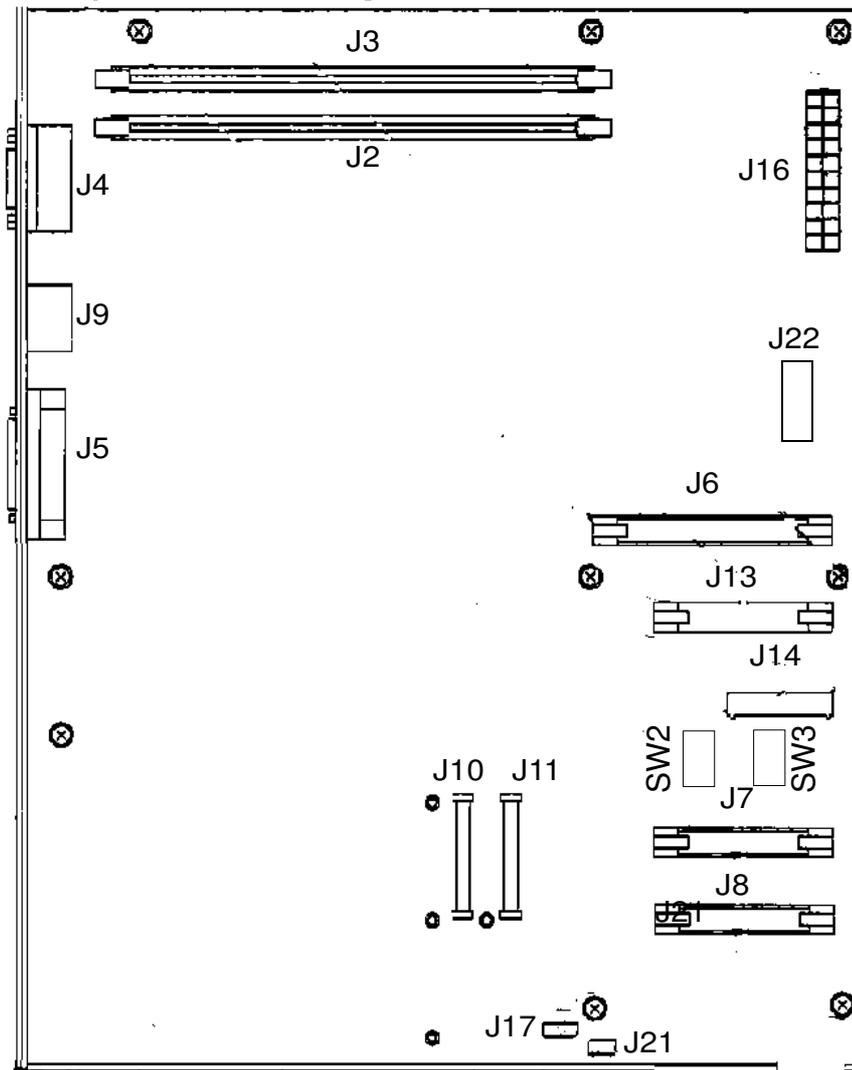
**Figure 5-5. Controller Board Layout**
