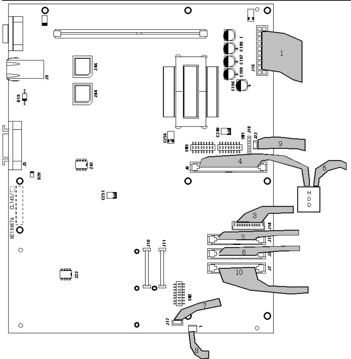
**Figure 5-3-1. Controller Internal Connections (CL143/CL144)**
