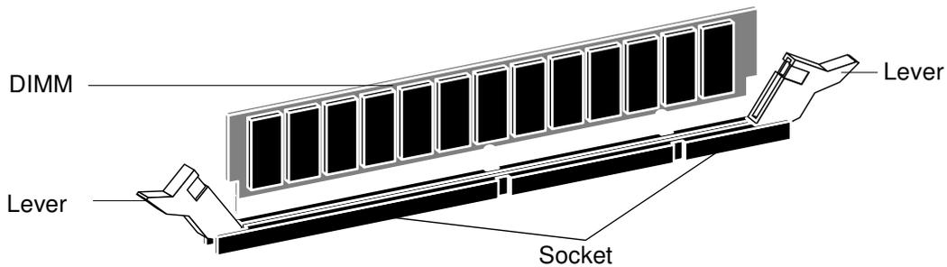
**Figure 5-8. Releasing a DIMM**
