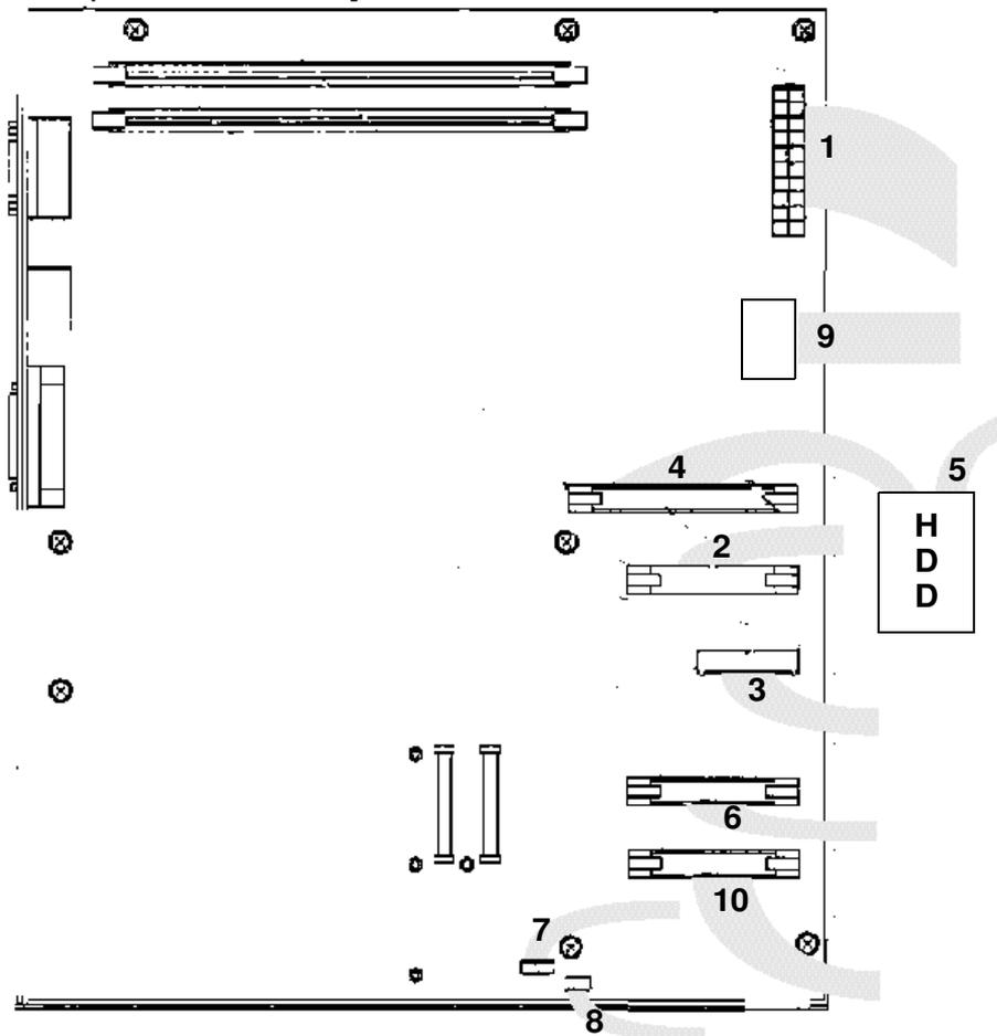
**Figure 5-3. Controller Internal Connections (CL106/CL107)**
