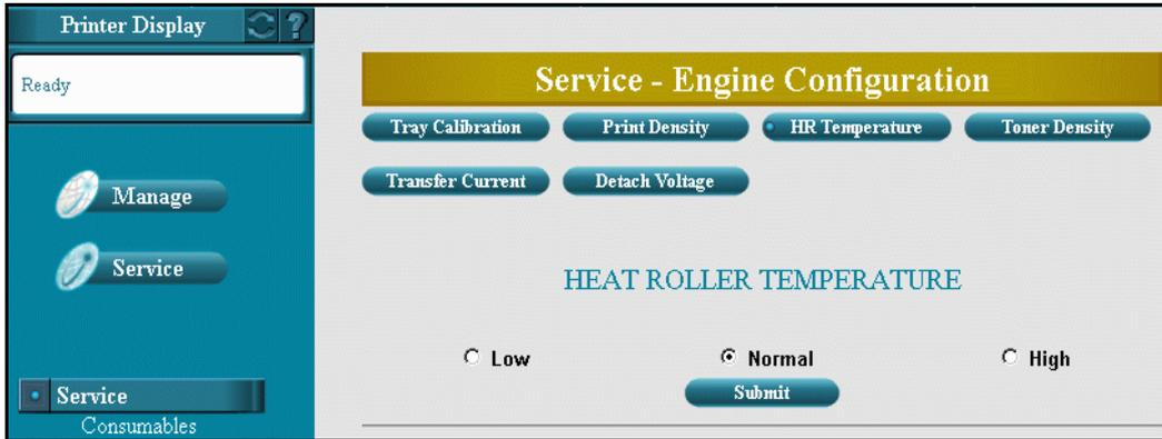
The HR Temperature value can alternatively be set using the Maintenance Panel. For information on the Maintenance Panel and this engine configuration setting, please refer to DDP Engine Maintenance Manual.
