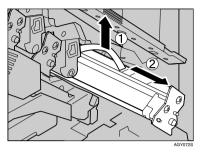
Install the new photoconductor unit. Take the unit out of the bag. For black, install one, and for color, install all three.
