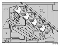
Remove the photoconductor unit you want to replace. Move the green hook slowly to the right, as shown. The green hook is located on the upper right of the photoconductor unit.
