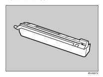
Hold the photoconductor unit, remove the adhesive tape from the end of the unit (1), and then remove the cap (2).
