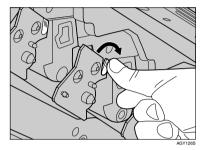
Phold the hook down, grip the green areas at the top and bottom of the photoconductor unit, and then slowly pull the unit out until you can see the entire green handle.
