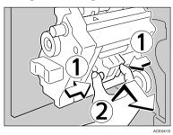
4 Hold both sides of the cartridge, and then pull up the upper unit of the cartridge.
