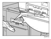
If the duplex unit is installed, close the duplex reversal unit.
