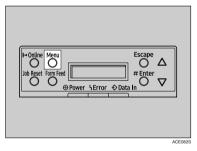
Press the [▲] or [▼] key to display "Maintenance", and then press the [# Enter] key.
