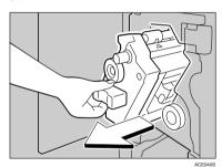
2 Hold the lever, and then pull out the staple unit.
