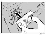
Plug in the power cable, and then turn on the power.
