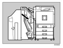
2 Pull out the punch waste box, and then remove the paper chips.
