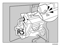
4 Push the cartridge button, and lift up while removing.
