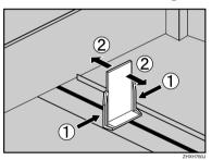
4 Align all four sides of the paper stack, and then load it in the tray.
