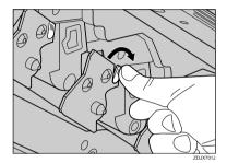
2 Hold the hook down, grip the green areas at the top and bottom of the photoconductor unit, and then slowly pull the unit out until you can see the entire green handle.
