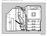
2 Remove the cartridge by pulling the green knob in the direction of the arrow.
