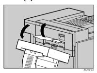
Slowly raise the duplex reversal unit and insert until it clicks into place. Raise the left cover, and then close it securely by pushing the area labeled "PUSH".
