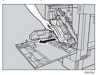
6 Hold the duplex feed unit using both hands, place it on the vertical rail, and slide it straight out.
