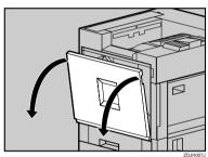
Carefully pivot the waste oil bottle outward, in the direction of the arrow.
