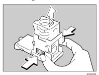
**5** Remove the empty refill in the direction of the arrow.
