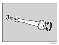
By pushing the screw into the screwdriver, you can work without having to worry about dropping the screw.
