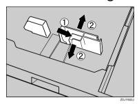
Adjust the end guide according to the size and orientation of the paper by gripping both edges of the guide (1), and then moving it in the direction of the arrow (2).
