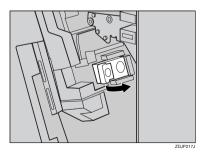
Open the cartridge face plate to unlock it.
