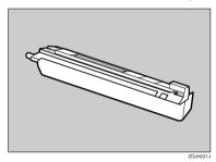
2 Hold the photoconductor unit, and remove the adhesive tape at the tip of the unit.
