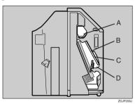
Check area A of step 4. Lift the lever (①), and then while holding it up with your hand, slowly pull out the misfed paper.
