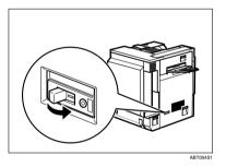
**5** Reset the earth leakage breaker by moving it to the "-" position.
