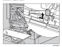
2 Insert the screw into the screw-driver.
