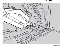
☐ Be sure to return the provided screwdriver to its original position on the inside of the front cover.
