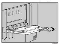
2 Slide the side guides outward (①), and then load paper print side up, until it stops (②).
