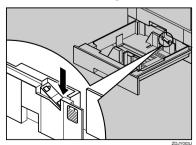
Press the side guide green lever (1), adjust the position of the guide by moving it in the direction of the arrow (2).
