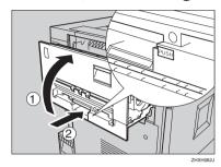
If you removed the external tray in step 4, reattach it to the printer. Insert the hooks of the external tray into the printer slits, and lower it toward you.
