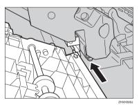
Refasten the duplex feed unit using the provided screwdriver. Use the screw removed in step 4.
