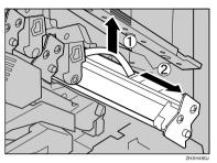
Install the new photoconductor unit.
