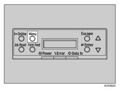
**2** Press the **[▲]** or **[▼]** key to display "Sample Print", and then press the **[# Enter]** key.
