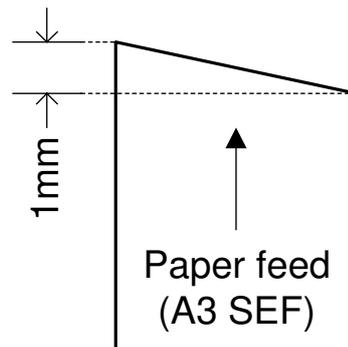
**Laser Beam Pitch Adjustment**
