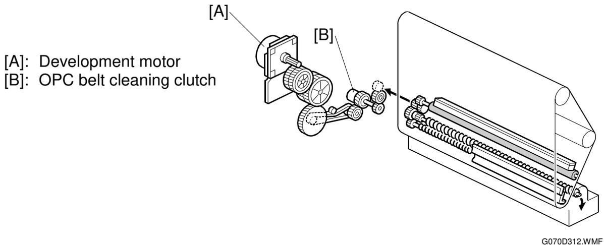
While the development motor is operating, the OPC cleaning clutch is always on. The clutch cuts the drive to the cleaning unit when the development motor reverses (this is done at intervals to prevent toner blockages in the development unit).
