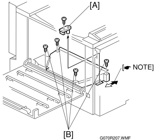
**NOTE:** When the image skews as shown, move the unit 1 mm in the direction of the black arrow as shown in the **upper** diagram.
