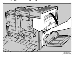
The fuser oil unit is placed on the fusing unit shown in the illustration.
