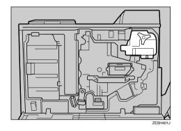
6 Release the green screw that is fastening the fusing unit.
