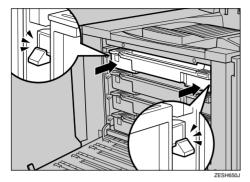
When there is a white line showing at the stoppers, reinsert the unit by following step **7**.
