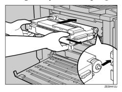
The illustration shows how to install the black development unit. The procedure is the same for all four colors.
