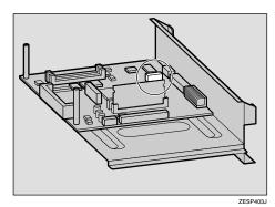
**7** Set the Account Enhance Unit on the controller board in the direction shown in the illustration.
