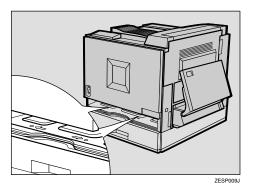
Use a coin to fasten them tightly. To connect two Paper Feed Units, fasten the two screws (for the front) as shown in the illustration.
