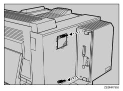
The removed screws will be used in step **(1)** to fasten the controller board.
