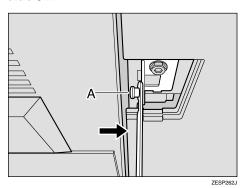
Attach one of the stoppers over the bar to fix the bar securely.
