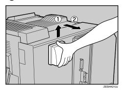
Remove the other dustproof filter cartridge by lifting it up.
