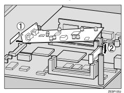
Confirm that the 1394 Interface Unit is firmly connected to the controller board.
