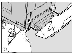
8 Align the projections and dents on the Duplex Unit and the printer, and then slide the Duplex Unit to the right until it clicks into place.
