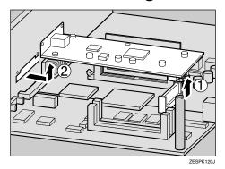
9 Set the 1394 Interface Unit on the controller board. Insert one end of the unit to the slot (①), and then connect the other end to the controller board (②).
