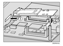
Confirm that the 802.11b Interface Unit is firmly connected to the controller board.
