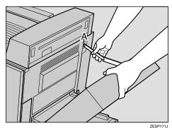
Connect the bar firmly by pushing it to the right as shown in the illustration.
