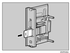
Adjust the controller board to the top and bottom rails, and then push in slowly until it stops.
