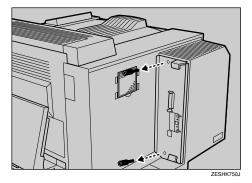
The removed screws will be used in step 11 to fasten the controller board.
