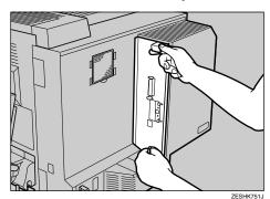
The Printer Hard Disk is to be installed on the back of the controller board.
