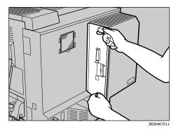
There are two slots for the Memory Unit. Use the available slot (the one in the front in the illustration) to install an optional Memory Unit.
