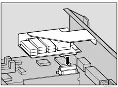
Confirm that the Account Enhance Unit is firmly connected to the controller board.
