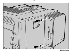
The removed screws will be used in step **(E)** to fasten the controller board.
