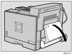
Extend the supporting bar on the Duplex Unit, and then connect it to the metal fitting (A) that has been attached to the printer.
