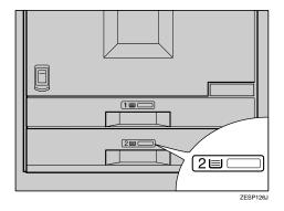
☐ After finishing installation, you can check whether the Paper Feed Unit is installed properly. Print the configuration page from the "List/Test Print" menu. If it is installed properly, you will see "Tray 2" or "Tray 3" under the "Options" list.
