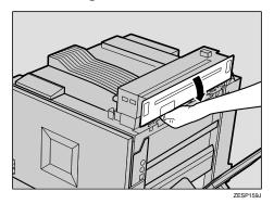
**3** Press the two projections on the Interchange Unit so that they securely fit into the holes of the printer.
