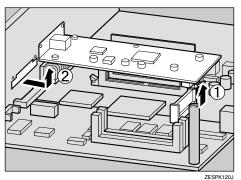
Attach the 802.11b Interface Unit. Insert the end of the 802.11b Interface Unit to the opening (①), and then push down until it clicks (②).
