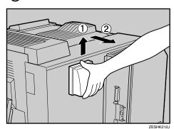
**4** Remove the other dustproof filter cartridge by lifting it up.
