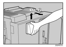
4 Remove the other dustproof filter cartridge by lifting it up.
