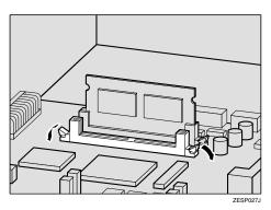
Adjust the notch of the Memory Unit to the slot, and then insert vertically.
