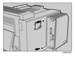
The removed screws will be used in step **1** to fasten the controller board.
