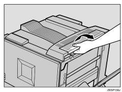
2 Press the cover to the right (1), and then lift the left edge (2) to remove it from the printer.
